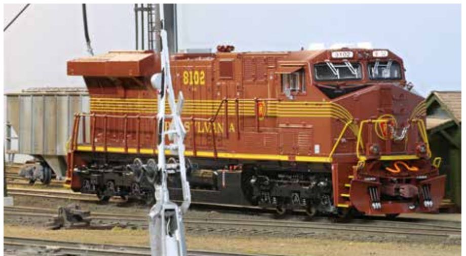
Bill Lane prepared this S scale Norfolk Southern Pennsylvania RR heritage unit from a Lionel S scale model. All that was required was to swap in scale wheelsets (available from Lionel) and install scale couplers. The paint and details on this DCC- and sound-equipped road unit are stock. Bill Lane photo
