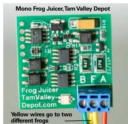
Fig. 5 Mono Frog Juicer. This Tam Valley Depot product controls frog polarity in installations where a turnout with auxiliary switching contacts are not used.
