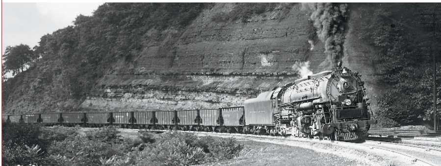
Sand on the rails and the smoke plume from the 2-8-8-4 show what hard work was required to lift Baltimore & Ohio coal trains up the 2.4 percent Cranberry Grade at Terra Alta, W.Va. Gordon R. Roth photo
