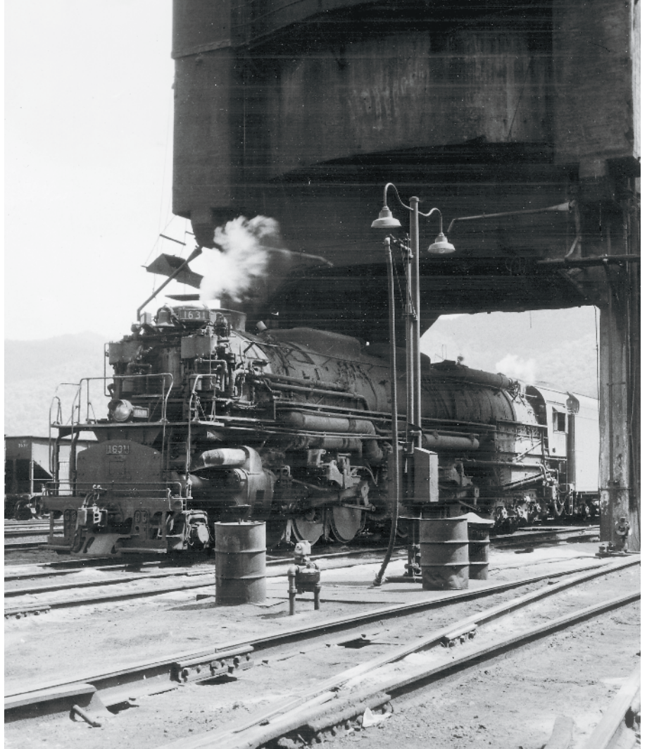
Hinton had a large engine terminal. In this photo, C&O 1631, a class H-8 Allegheny, takes on sand at the sand house. Wayne Carman photo
