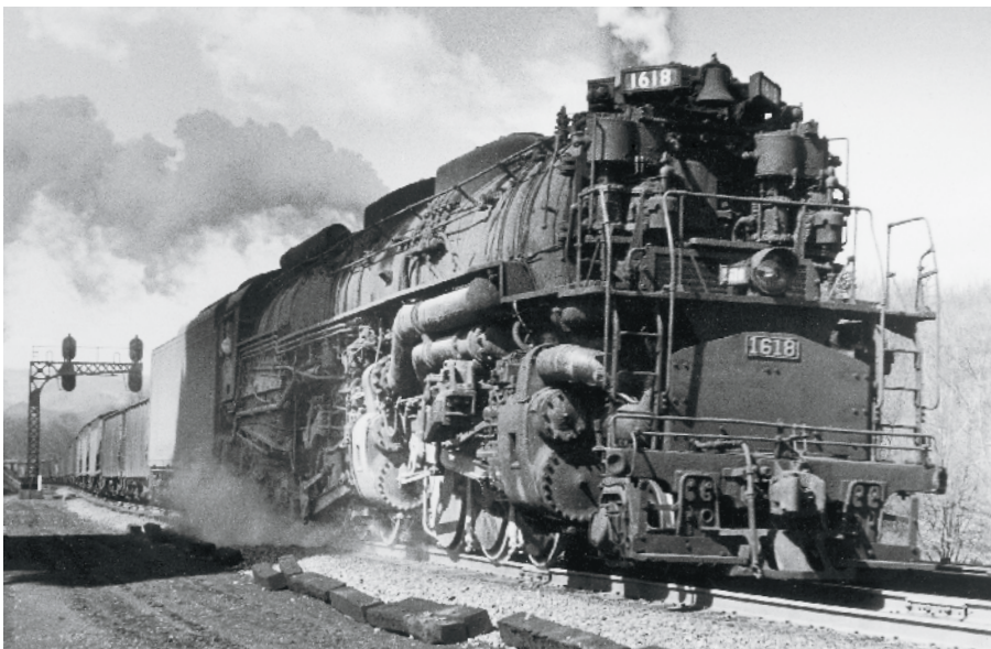
Near White Sulphur Springs, W.Va., in 1953, class H-8 2-6-6-6 no. 1618 pulls a coal drag upgrade toward the summit at Allegheny. Parker Hayden photo
