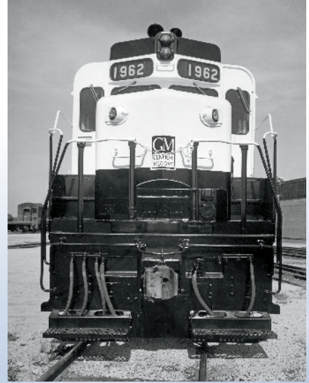
Electro-Motive's 2,250-hp GP30 is billed as a combination "high speed and heavy drag" locomotive, a pair of which can replace three older 1,500-hp units. EMD
