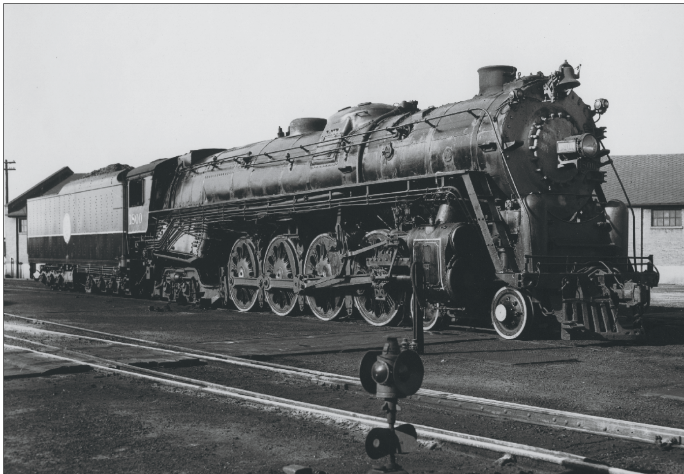
The ultimate development of dual-service power on the Atlantic Coast Line was the R-1-class 4-8-4, built by Baldwin in 1938. In appearance the R-1s were very much the modern Baldwin locomotive. Trains collection
