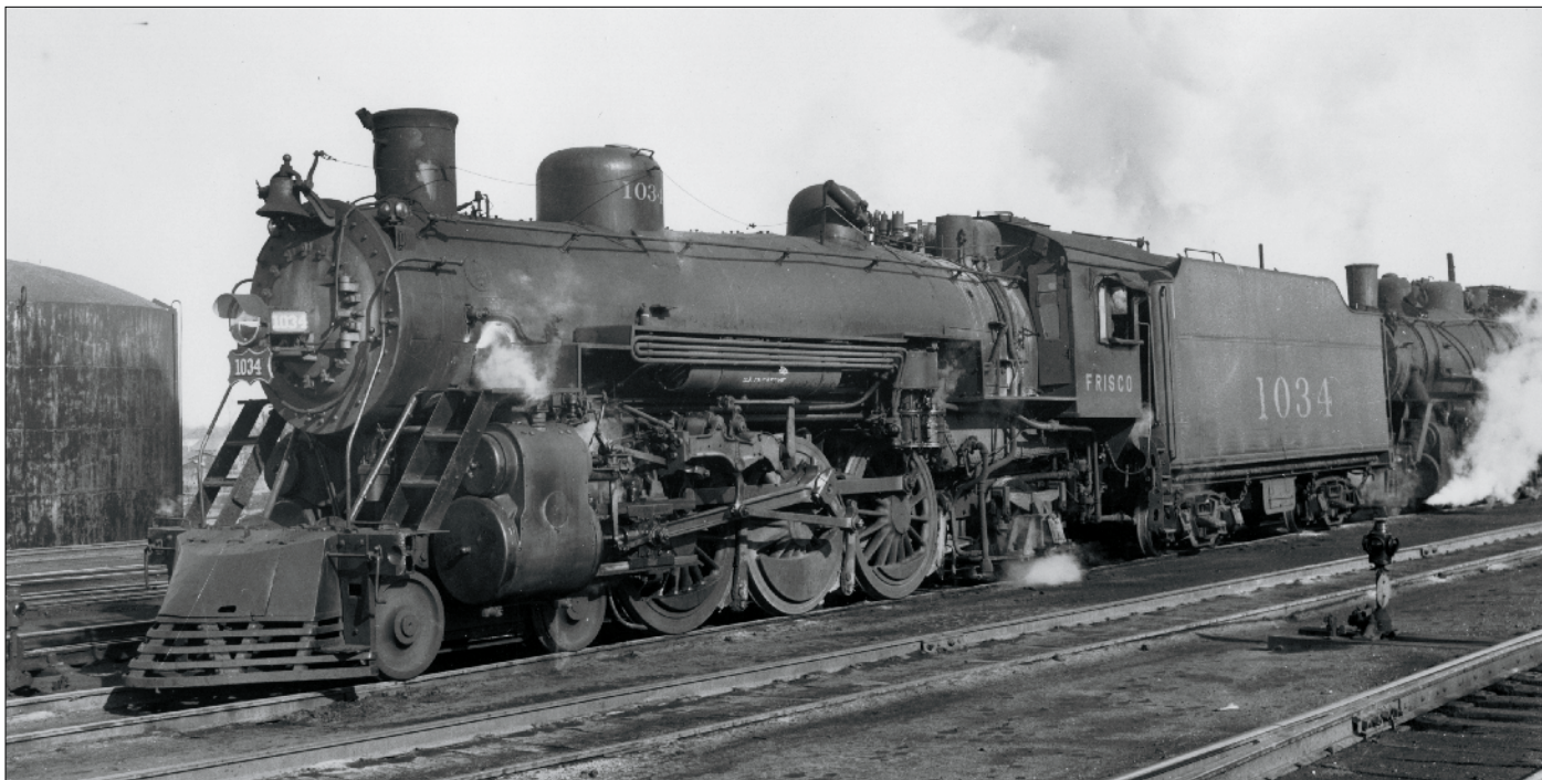
The 4-6-2 Pacific was the dominant type of passenger locomotive in North America for most of the early 1900s. Here St. Louis-San Francisco no. 1034, built by Baldwin in 1910, is on the ready track at Springfield, Mo., in December 1948. Arthur B. Johnson
