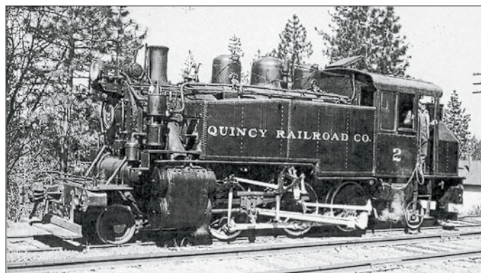
Tank engine — Quincy no. 2, an Alco product of 1924, carried enough water in its side tanks and fuel oil in the rear tank for the 6-mile run between Quincy, Calif., and the connection with the Western Pacific at Quincy Junction. Guy L. Dunscomb
