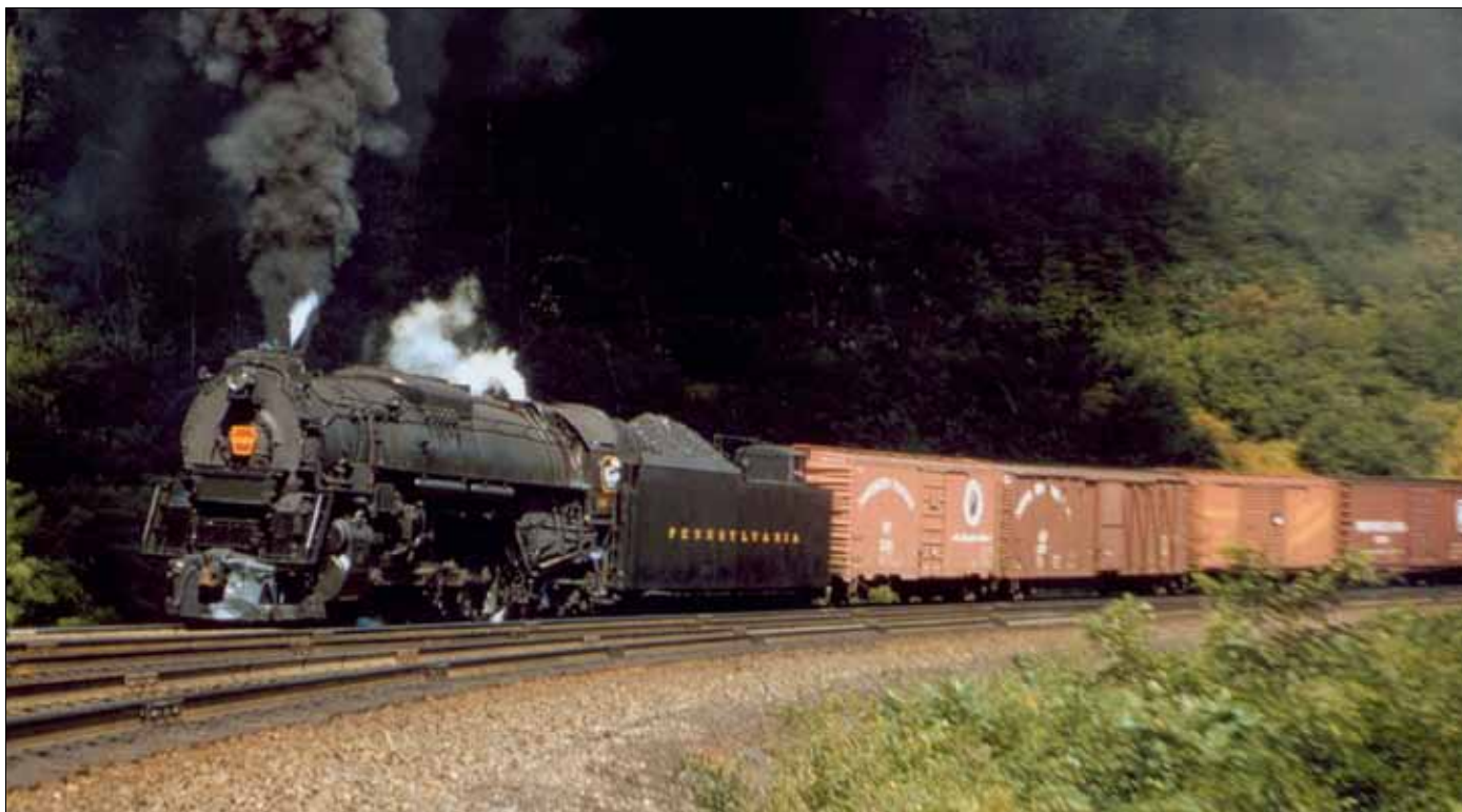
A Pennsylvania J1-class 2-10-4 lugs a freight upgrade on Horseshoe Curve, arguably the railroad's most-famous landmark, in 1955. Pennsy had 125 of the big Texas-type locomotives, more than any other railroad. Bob's Photo
