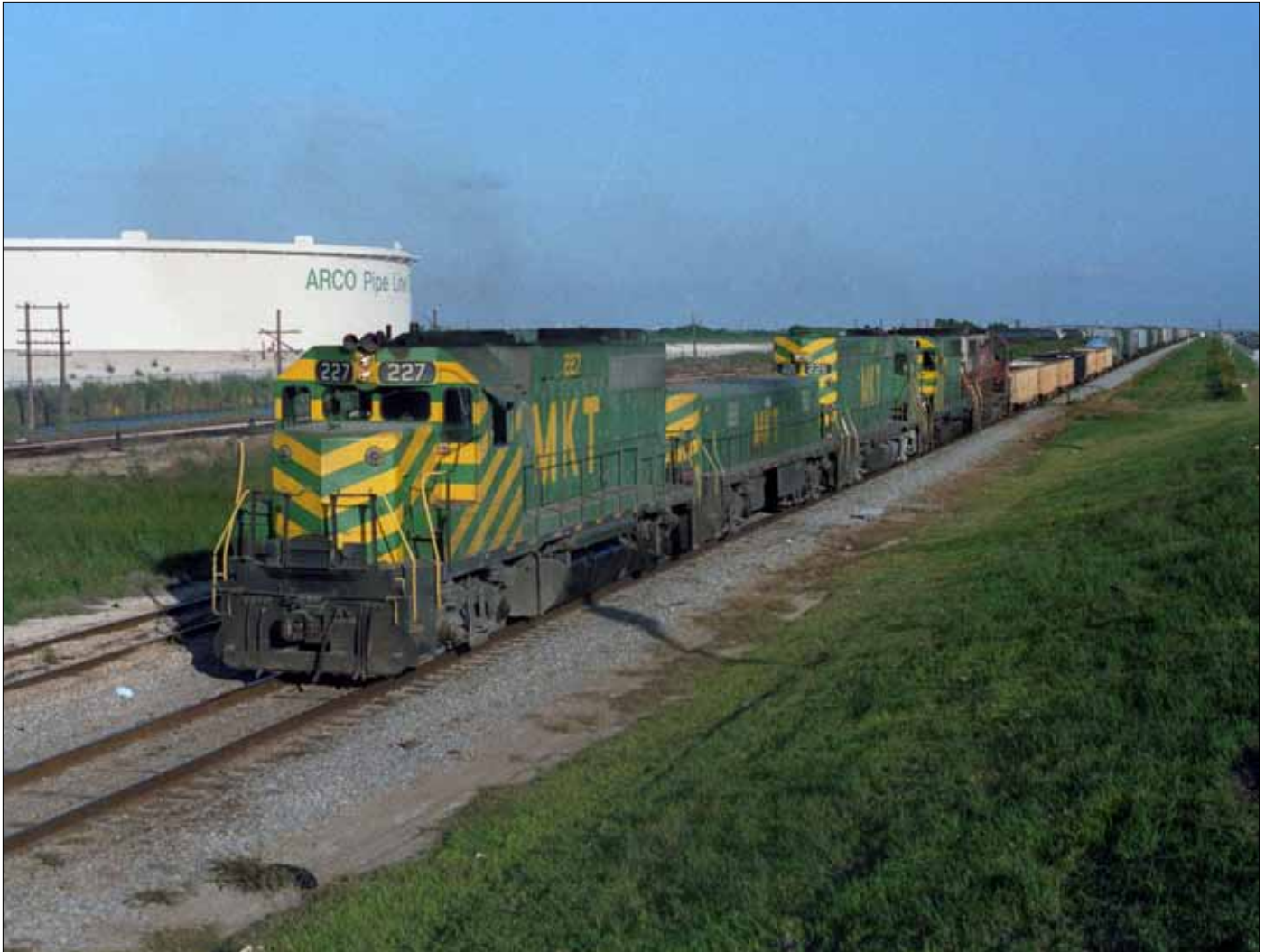
A northbound freight, with a GP40 leading and a slug immediately behind, heads out of Texas City, Texas, along the sea wall. The tank farm is owned by Arco Pipeline (now BP). Note that the trailing locomotive is in Katy red in this July 1988 view. Laurence Pearlman
