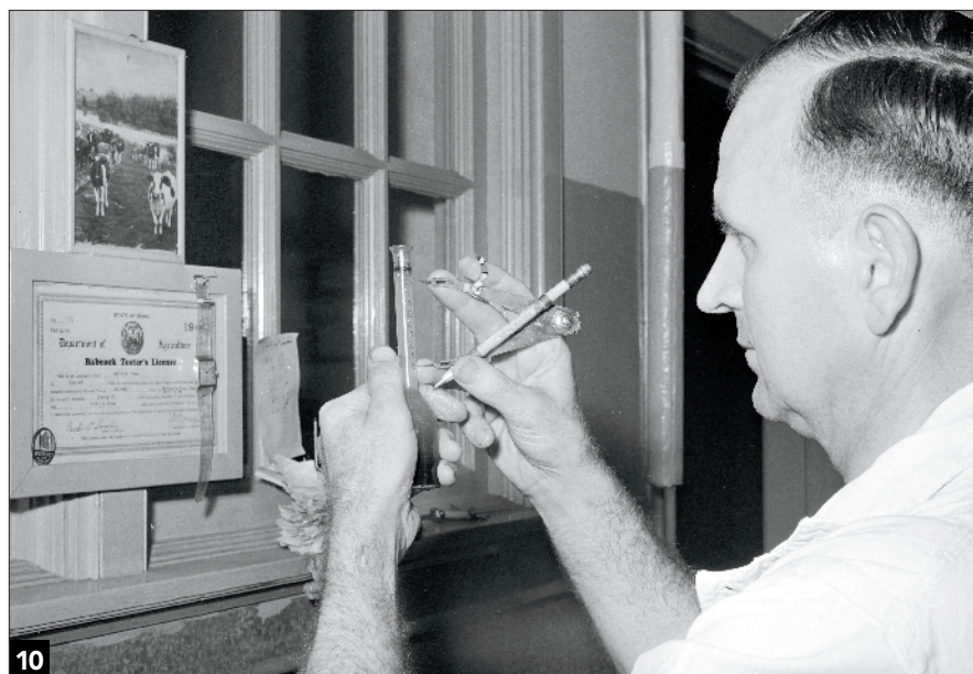
The Babcock test was developed in the 1890s. It is a simple, accurate method of measuring butterfat content by adding sulfuric acid to a milk sample. Russell Lee, Library of Congress
