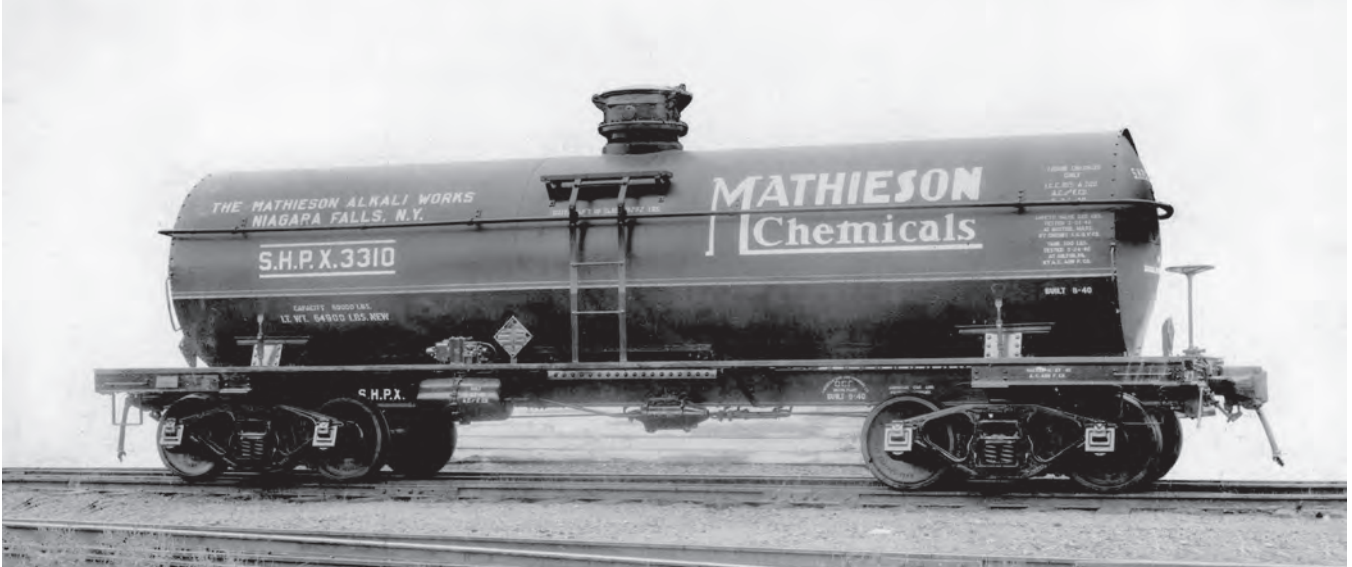
Mathieson Chemicals leased this chlorine car from Shippers Car Line. The 40-ton, ICC 105A 300 car was built by American Car & Foundry in 1940. American Car & Foundry
