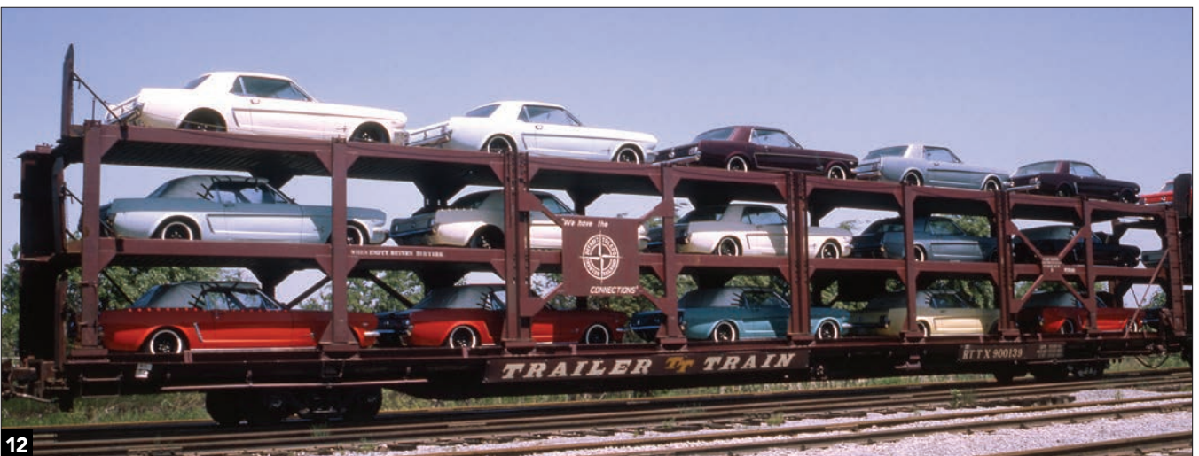
Fifteen new 1964 Ford Mustangs leave Detroit on RTTX 910546, an 89-foot tri-level open autorack. The rack is secured to the Trailer Train flatcar. Racks were owned by the railroads participating in pools of cars (in this case, Detroit, Toledo & Ironton). The automobiles are secured to the rack with chains built into the decks. J. David Ingles collection
