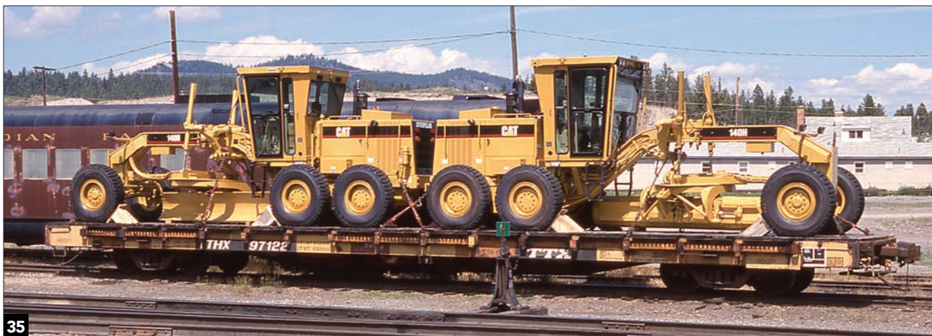
A pair of Caterpillar 140H graders have arrived on a TTHX car at Cranbrook, B.C., in June 2001. Heavy chains and blocking secure the load to the deck. The blades rest on 2x4 blocks and are chained to keep from rotating. Keith Kohlmann
