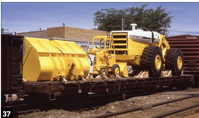
This THX car has just been pulled from the Hough factory in Libertyville, Ill., on June 11, 1972, by the Milwaukee Road switch crew. The load at right is a model 560 Payloader, a 40-ton machine with a 6½-cubic-yard bucket. The company's much-smaller model H-25 Payloader (middle) has a ½-yard bucket. There is about a 15-year difference in technological development between the two designs.
