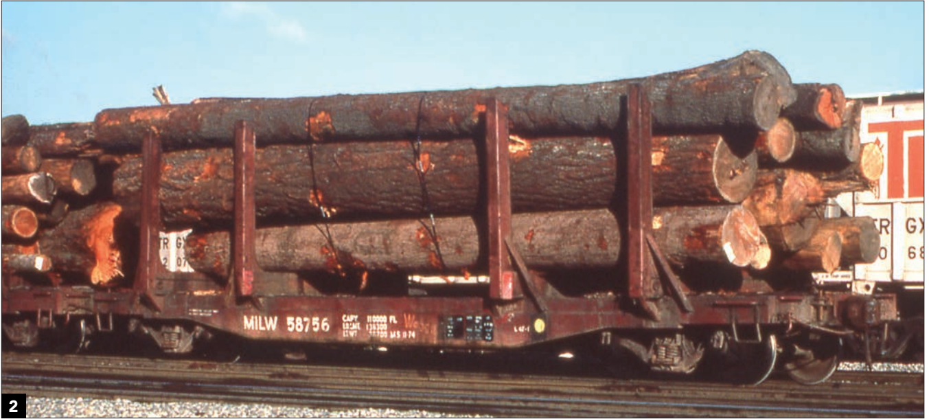
2 This Milwaukee Road log flatcar carries 11 logs to a sawmill in 1978. This modern, 42-foot, welded all-steel car was built for this purpose. Heavy stakes support the logs, which rest on large steel bunks. This arrangement allows the car to be loaded and unloaded by a wheel loader equipped with forks and a grapple. Steel banding keeps the load from shifting. Paper tags help identify the load at the mill. Keith Kohlmann collection
