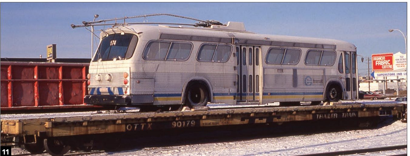
Edmonton Transit Service no. 174 is a Brown Boveri electric bus that has returned to Edmonton after being on loan to the Toronto Transit Commission. It's riding on an OTTX flatcar and spotted at the team track ramp in Strathcona Yard at South Edmonton, Alberta, in December 1993. The bus is riding low because its air suspension has been drained for the cross-Canada journey. The wheels are blocked and the bus is chained down. Keith Kohlmann
