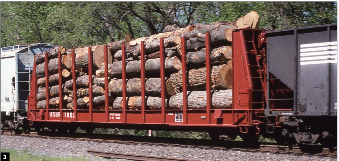
3 This modern 100-ton capacity bulkhead flatcar carries a full load of hardwood logs at Sunbury, Pa., in May 2002. The car has permanent side stakes with five chains running across the top of the load. Ruben S. Brouse
