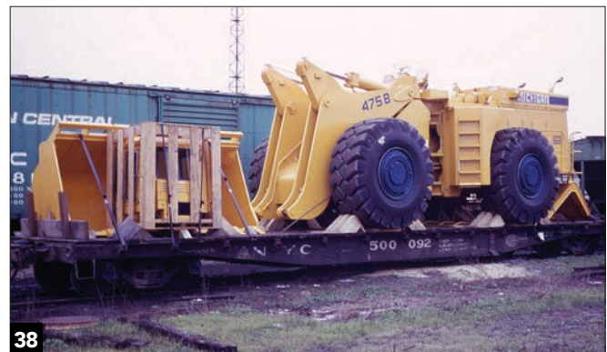
A Clark Equipment Co. Michigan 475B articulated wheel loader fits on a New York Central flatcar at Sharonville, Ohio in April 1973. The bucket and all parts above the driver's compartment have been placed onto the deck so the load can meet clearance limits. The cab, railings, and roll-over protection cover are blocked, nailed, and strapped to the car. The load is as tall as the adjacent boxcar.
