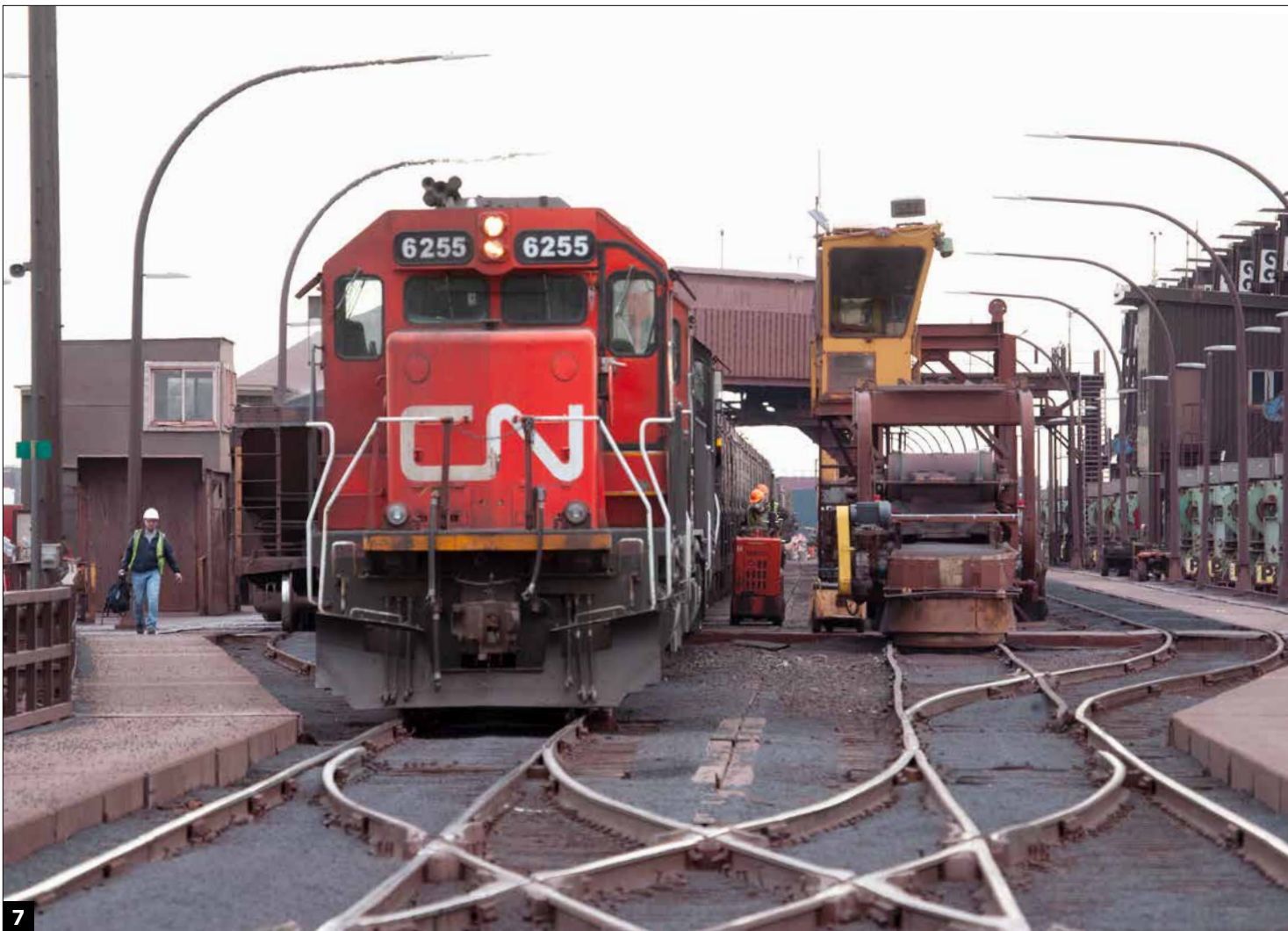
A taconite pellet train has just arrived for unloading at the Canadian National (former DM&IR) Duluth dock no. 6 in April 2015. A double crossover allows access to all four dock tracks. Craig Williams
