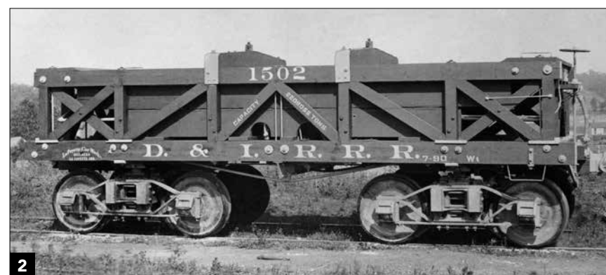
Right: Duluth & Iron Range 1502 is a 22-ton wood car built by LaFayette Car Works in 1890. It has archbar trucks and link-and-pin couplers. Trains magazine collection
