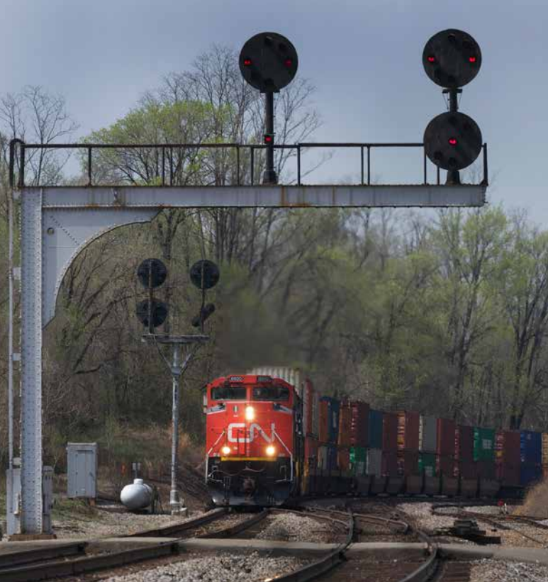
Signal heads on the famous Norfolk & Western Blue Ridge Grade east of Roanoke, Va., are installed so as to only be able to show possible aspects through the single crossover in the interlocking. Norfolk Southern train 236 is behind Canadian National power in 2014.
