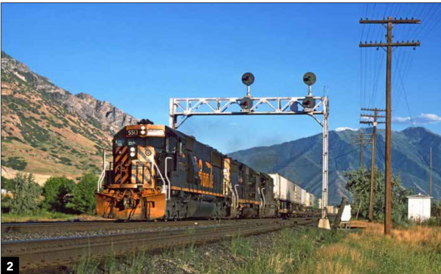
Signals come in many different shapes and sizes, and are mounted in different ways. Here, GRS searchlights are mounted on a bridge over the Rio Grande main line through Ironton, Utah. James Belmont
