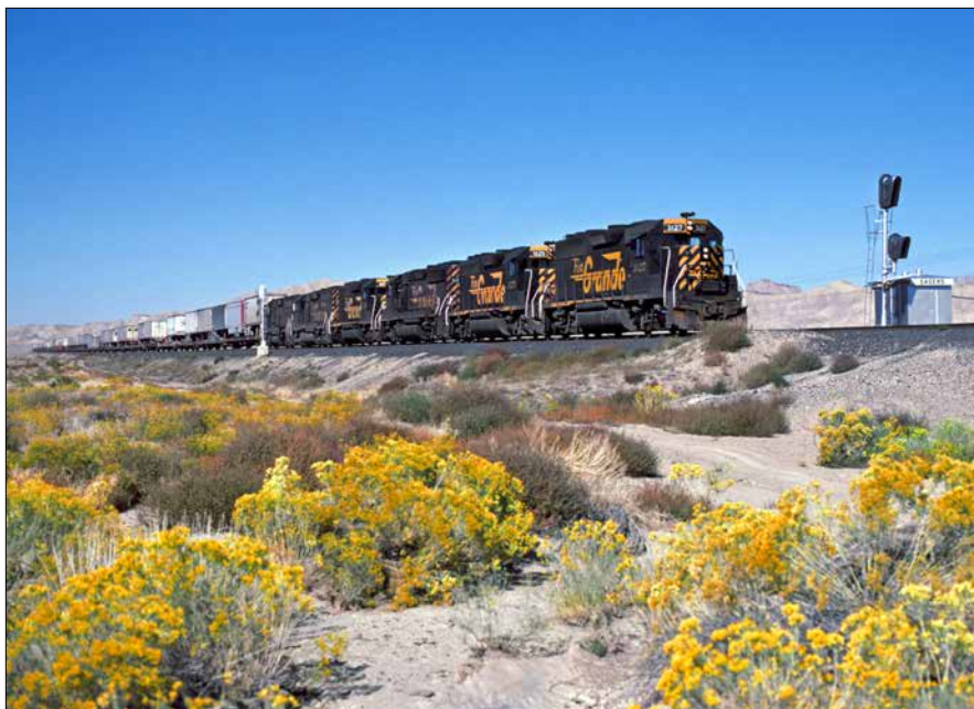
Rio Grande train No. 100 races eastward across Utah's desolate Green River Desert and passes into the interlocking at East Sagers, Utah, the morning of Oct. 2, 1987. The controlled siding at Sagers is protected by GRS Type D signals, which were common on the Rio Grande. James Belmont.
