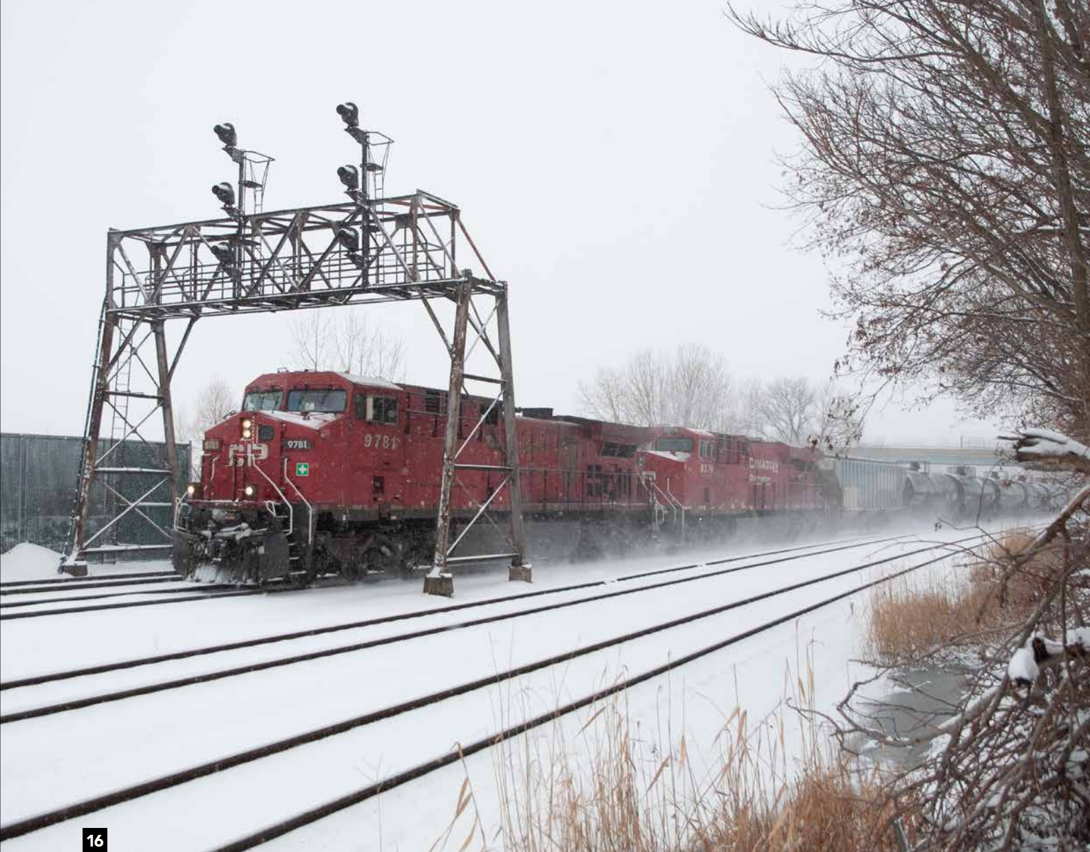
Canadian Pacific AC4400CW 9781 leads oil loads under the unique modified signal bridge at CP 286 in East Syracuse, N.Y., in 2014. Railroads modified the original signal structures as needed when tracks were moved or as operational changes required. This bridge is the prototype for the bridge holding the eastward home signals at CP 280 on my Onondaga Cutoff.
