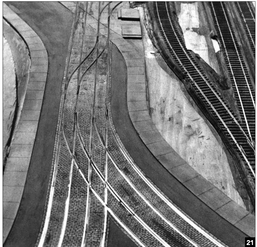
Walt carved bricks only along the tracks, keeping the outside rows parallel to the rails. The bricks have a realistic, slightly uneven look. The layout is the HO scale Brandywine Transit Co. Walter R. Olsen
