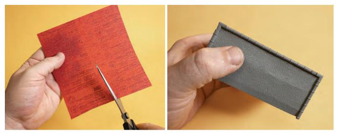
To help simulate the tar paper and gravel roof, I used a sheet of 120 grit sandpaper cut to size. I've come to prefer this material for modeling flat roofs, since it gives me more control and a better appearance than trying to use real rock or ballast. The sandpaper was painted with a dark gray spray paint primer, and glued to the top of the core with CA.
