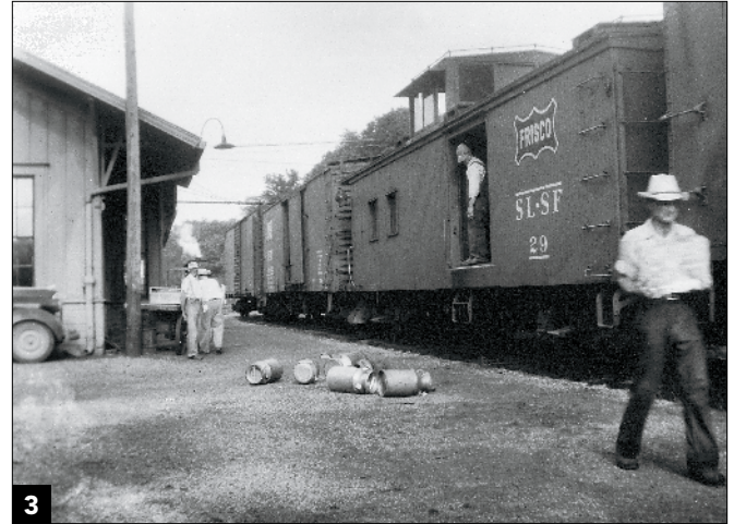
3 Some railroads used side-door cabooses to carry LCL on branch lines. Here, the St. Louis-San Francisco crew has just unloaded several empty milk cans at Steelville, Mo., in 1949. Frank Barry
