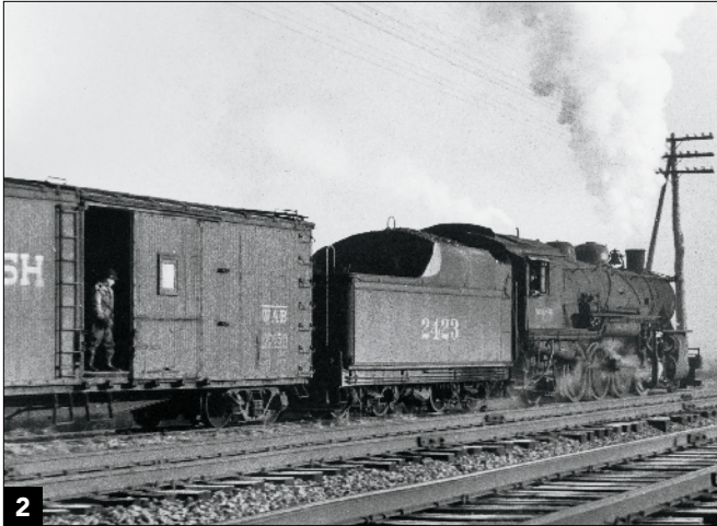
2 Peddler cars (or waycars) carried LCL to multiple stations along a route. Some were specially equipped and manned by messengers, as is this car on the Wabash at Marshfield, Ind., in 1948. Ralph E. Byers
