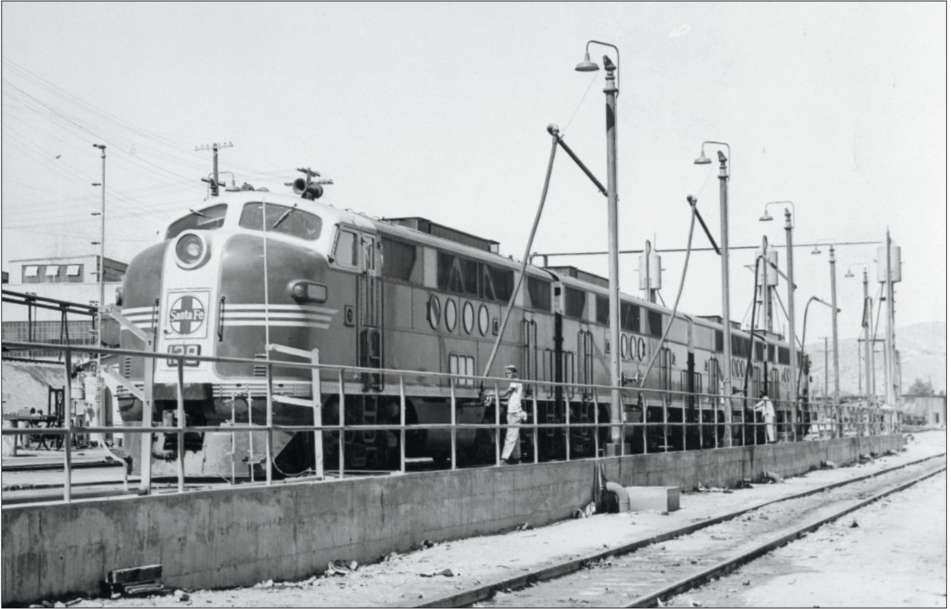
A four-unit set (5,400 total horsepower) of Electro-Motive FTs takes on diesel fuel at the fueling rack at Santa Fe's Barstow, Calif., shops. The tall tanks in the rear at right hold traction sand. Several locomotives can be fueled at once. Santa Fe Railway
