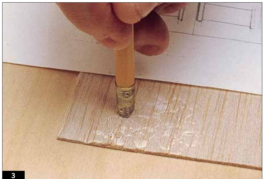
3 Push the pencil end squarely into the balsa, working diagonally from bottom to top in a checkerboard pattern. Turn the pencil as you work and overlap some previous impressions to vary the size and shape of the stones.
