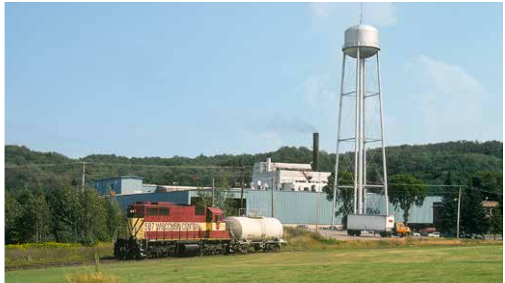
Local L042 works at Munising, Mich., on Aug. 27, 1990. EMD SDL39 No. 587 is one of 10 such lightweight, six-axle units built for the Milwaukee Road 1969-1972 for service on branch lines, often in Wisconsin.
