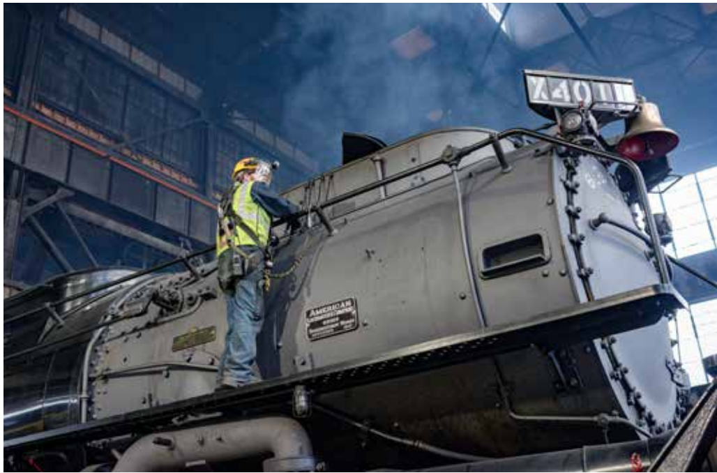
Maintaining No. 4014 is a constant regimen of following inspection schedules. The entire steam crew is involved in a hands-on manner so that everyone becomes familiar with the entire locomotive. Here the stacks and smoke deflectors are being examined.
