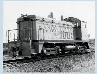
Union Pacific No. 1800 is a late SW7, indicated by the straight-top cab windows. The hood has the single taper at the cab of later SW-series locomotives. *EMD*
