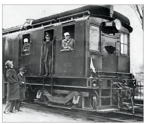
Long Island Rail Road No. 401, a 100-ton boxcab built by Alco/GE/Ingersoll-Rand, is often credited with being the first road diesel-electric in the U.S. Long Island Rail Road
