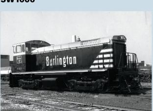
The SW1000 introduced a new cab design and higher-level running boards. *EMD*
