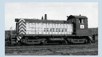
Weyerhaeuser No. 1 is an SW600. It has five slits on the battery-box louver behind the cab—but early models had six slits, like the SW8. *Stan Mailer*
