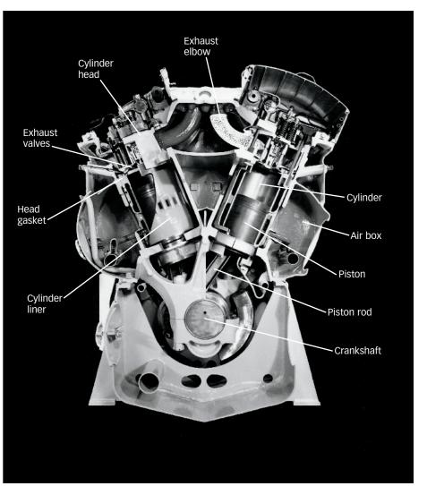
This cutaway cross-section view shows an Electro-Motive Division 567 diesel engine, a V-style design with cylinders at a 45-degree angle. EMD
