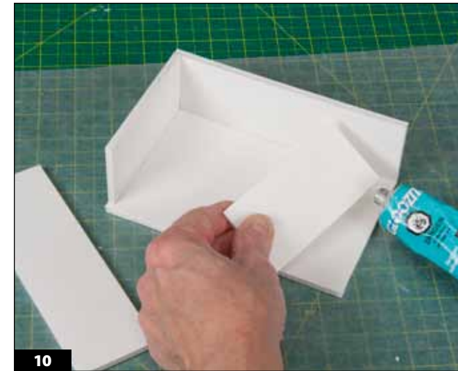
10 To assemble the foam core into a basement, you can use contact cement as well as model glue, rubber cement, or carpenter's glue.
