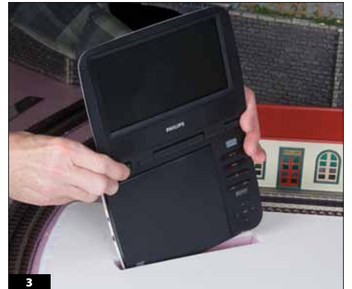
3 Test that the screen and additional components of the DVD player fit through the slot and function properly.
