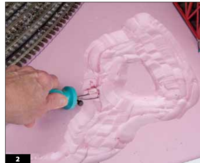
A round-tipped blade fitted to a hot wire tool makes it easy to carve out a shallow pond.
