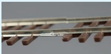
A piece of code 70 rail is soldered to the top of the flattened rail joiner.
