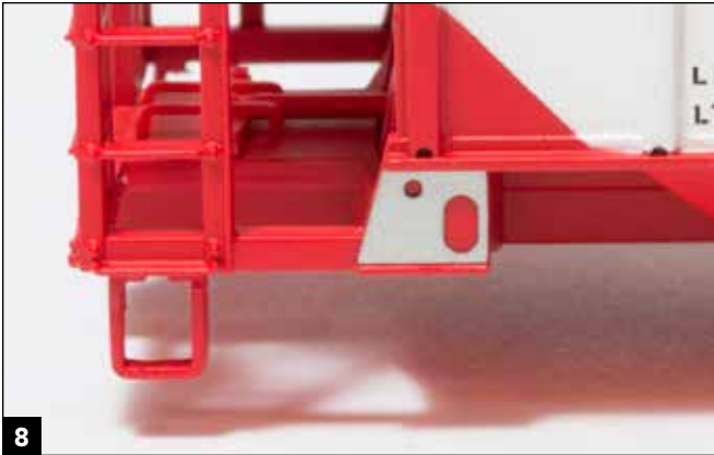
8 The roping holes were originally printed on the model. I used jack pad faces from a Plano kit to upgrade these areas.
