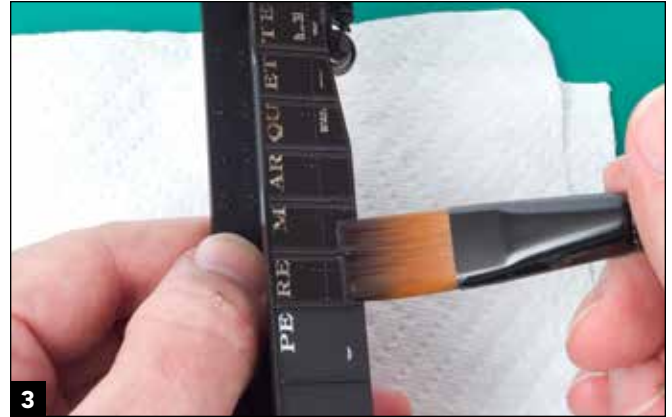
3 Weather the car with washes of rust-colored artist's oil paints, brushing them downward along each side panel.
