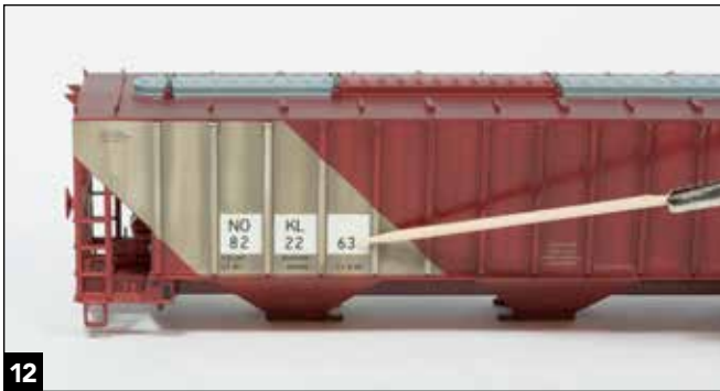
12 A decal set for center-beam bulkhead flatcars contains NOKL reporting marks and road numbers in a font that is similar (but smaller) than the one used on the full-sized covered hopper.
