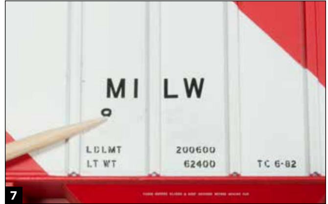
7 To avoid having to repaint the car, I used Microscale Micro Sol to remove unwanted graphics. I wet-sanded areas where the black printing left residue on the white and red paint with 600-grit and 1,500-grit sandpaper.
