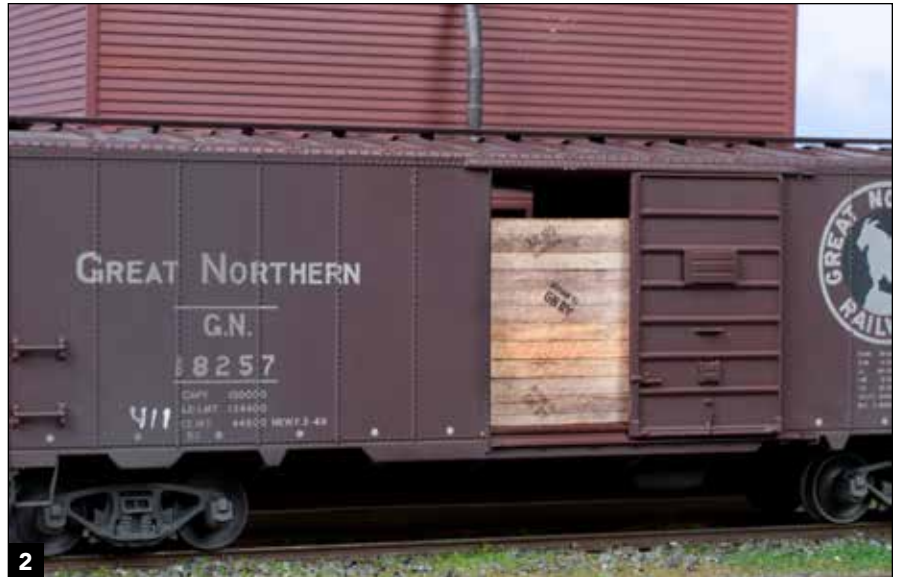
2 The printed grain doors are quite realistic, showing wood grain and weathering as well as stencils that indicate ownership. The boxcar is from InterMountain.
