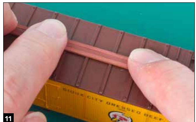
11 Press the new wood running board in place, making sure it's aligned properly.
