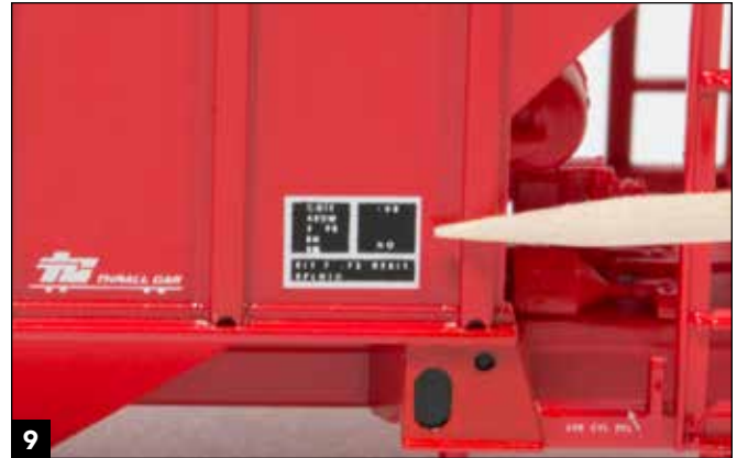
9 Microscale decal sets MC-5004 and 87-1276 provided the new COTS panel and Thrall builder's stencil, respectively.
