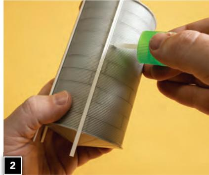
2 I then applied Plastruct styrene C-channel pieces to the sides to model the legs, 2. Six separate strips were attached evenly around the entire bin, and extended 2 inches below the bottom of the bin.
