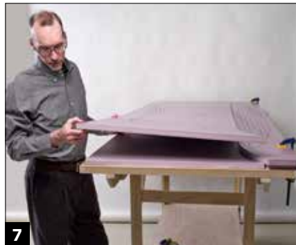
David Popp used two sheets of foam board for the surface of the layout, with the lower piece cut smaller to create a wiring recess.
