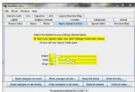
2. The Basic Speed Control pane in DecoderPro allows you to enter values for CVs 2, 5, and 6 either by keying them in or with the sliders.
