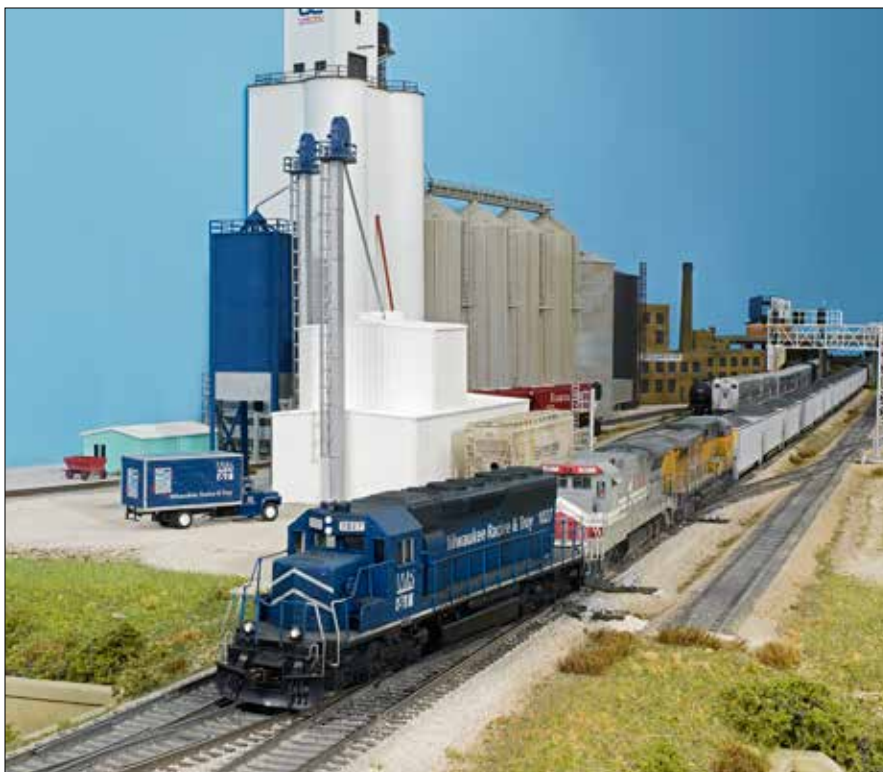
SD40-2 no. 1027 leads a unit coal train through Williams Bay on the Milwaukee, Racine & Troy club layout at the Kalmbach Media offices. Using DCC consisting you can operate multiple locomotives just as the prototype does.
