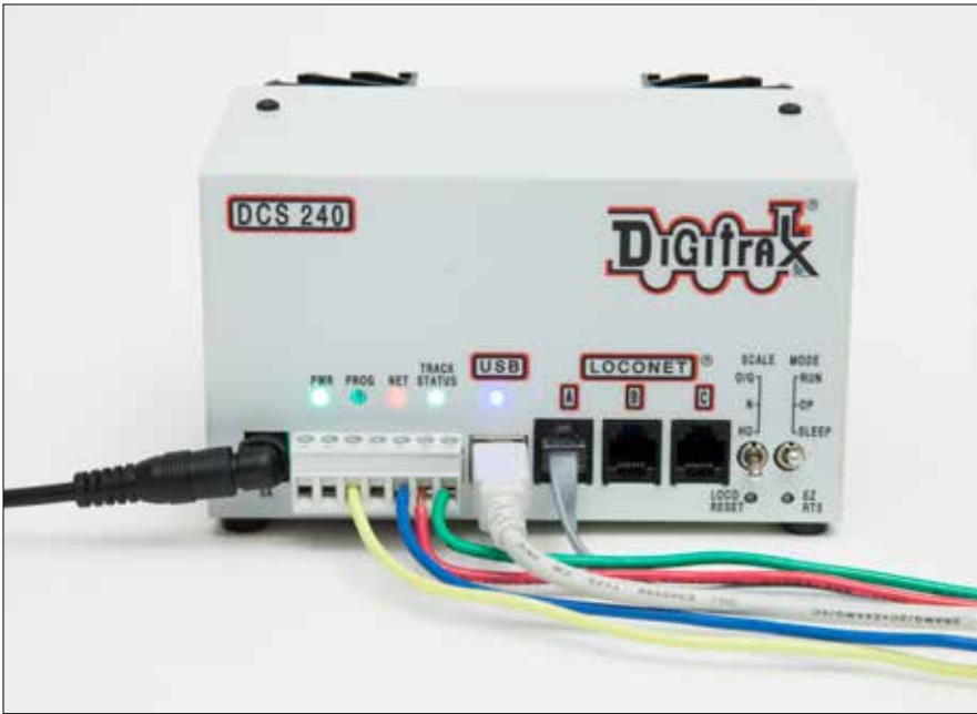
4. Digitrax began revamping its line of command stations in 2016 with the Digitrax DCS240. The system includes the addition of a USB port to allow a computer interface.
