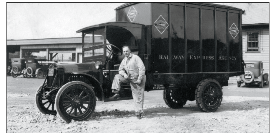
This early 1920s Diamond T shows the open cab and narrow tires typical of that era. It sports a fresh paint job in 1930 for Railway Express Agency. Jeff Wilson collection
