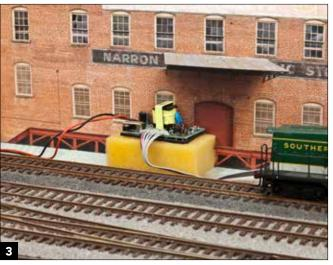
Mounting the circuit board on a piece of soft foam practically eliminates the high-frequency sound generated by the circuit.
