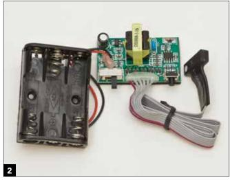
Each circuit board is attached to a battery pack that holds three AAA batteries. Boards have on/off and animationselection switches.
