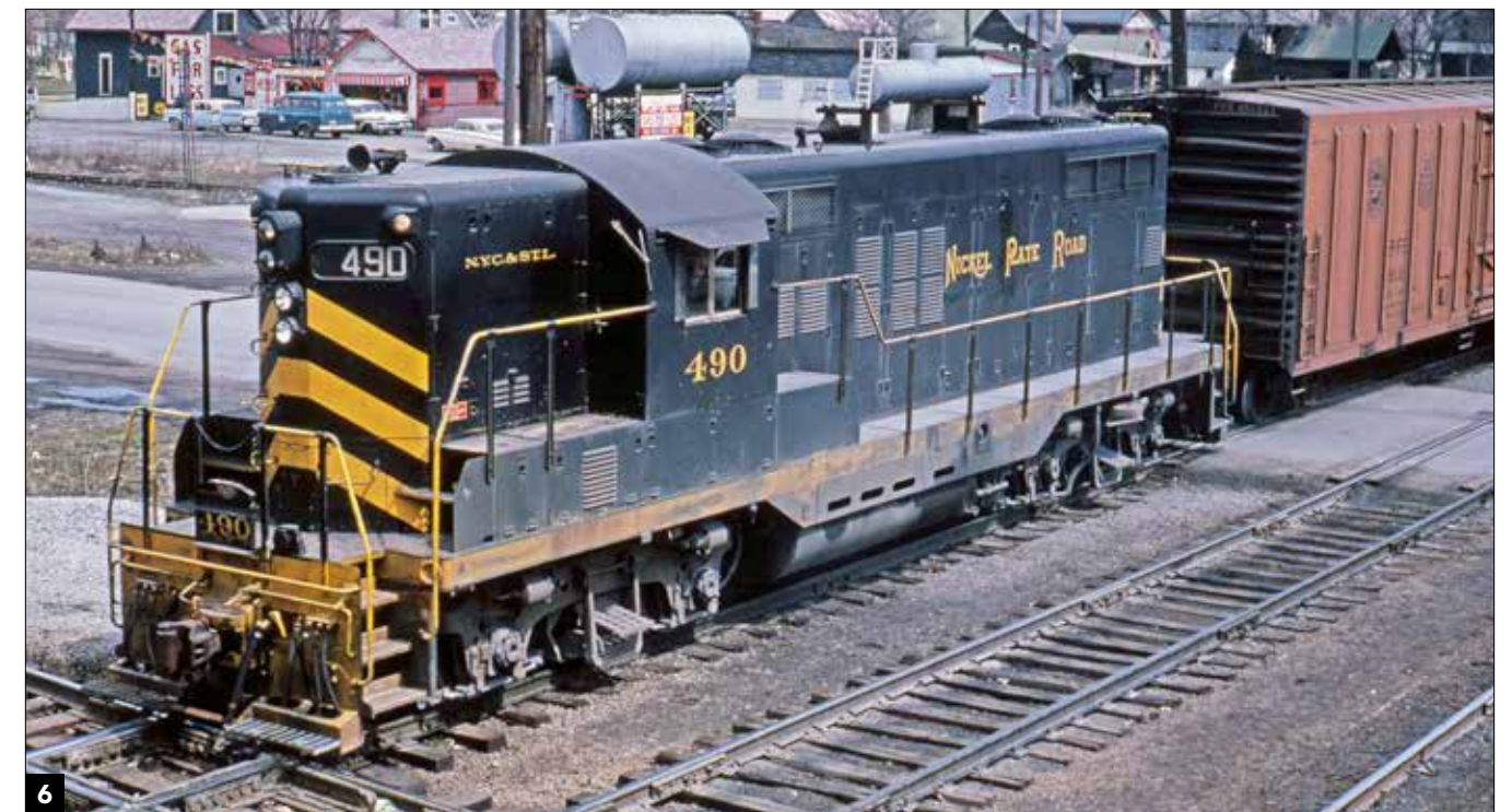
6 Dick Dilworth's utilitarian "Geep" debuted in late 1949. The carbody remained largely unchanged from the first GP7 until the introduction of the GP30 in 1961. Nickel Plate 490 is an early model GP9; note the four 36"-diameter rooftop fans (later GP9s had two 48"-diameter fans). GP7s also had two sets of louvers on the panels below the cab number. The NKP eschewed dynamic brakes. The unit has been repainted in the railroad's post-1959 wide-stripe scheme.
