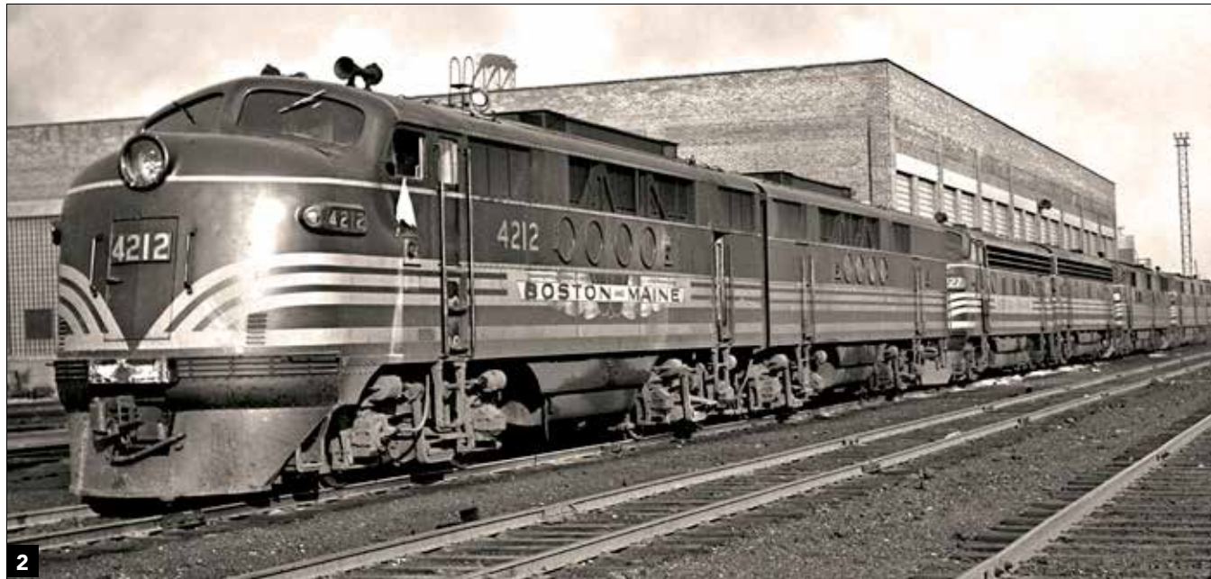
2 An A-B set of drawbar-connected Boston & Maine FTs (in Boston in March 1950) shows the distinctive four-porthole styling and close spacing between units. The boxy structure on the roof is the dynamic brake housing. The F unit's "bulldog" carbody styling blended nicely with passenger cars but did not facilitate clear views to the rear for en route freight-car switching. George Corey
