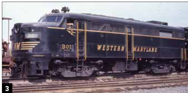
3 The blunt-nosed Alco FA was a dramatic improvement over earlier Alco cab-unit designs. Western Maryland 301 was one of four FA-2s on its roster. The vertical shutters on FA-1s are mounted farther back near the rear bulkhead.
