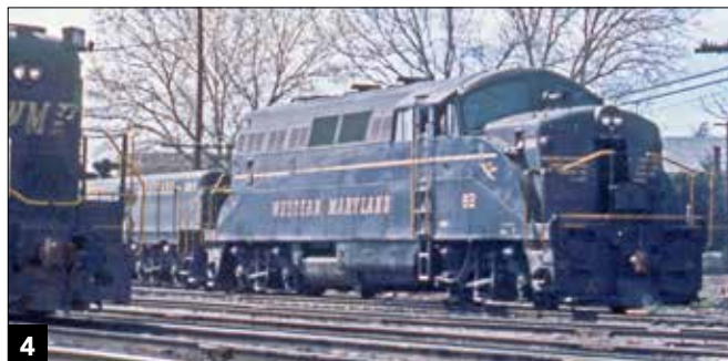
4 EMD's BL1 (only one was built) and BL2 were intended to provide greater visibility for switching branch lines. The rapidly growing popularity of the road switcher brought production to an end after 13 months. Western Maryland's two BL2s were later paired with "slugs" for switching in Hagerstown, Md.
