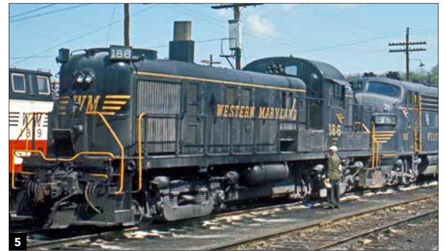
5 Alco followed the RS-1 with the 1,500-h.p. RS-2 (1946–50) and similar 1,600-hp RS-3 (1950–56); six-motor (RSD-4 and -5) and A1A (RSC-2 and -3) versions were also offered. WM 186 is an RS-3: Note boxes on frame fore and aft of the cab.
