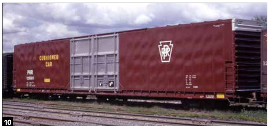
New 86-foot cars, designed to carry stampings and other lightweight parts, became common sights by the mid-1960s. This Pennsy car was built by Pullman in 1966. J. David Ingles collection
