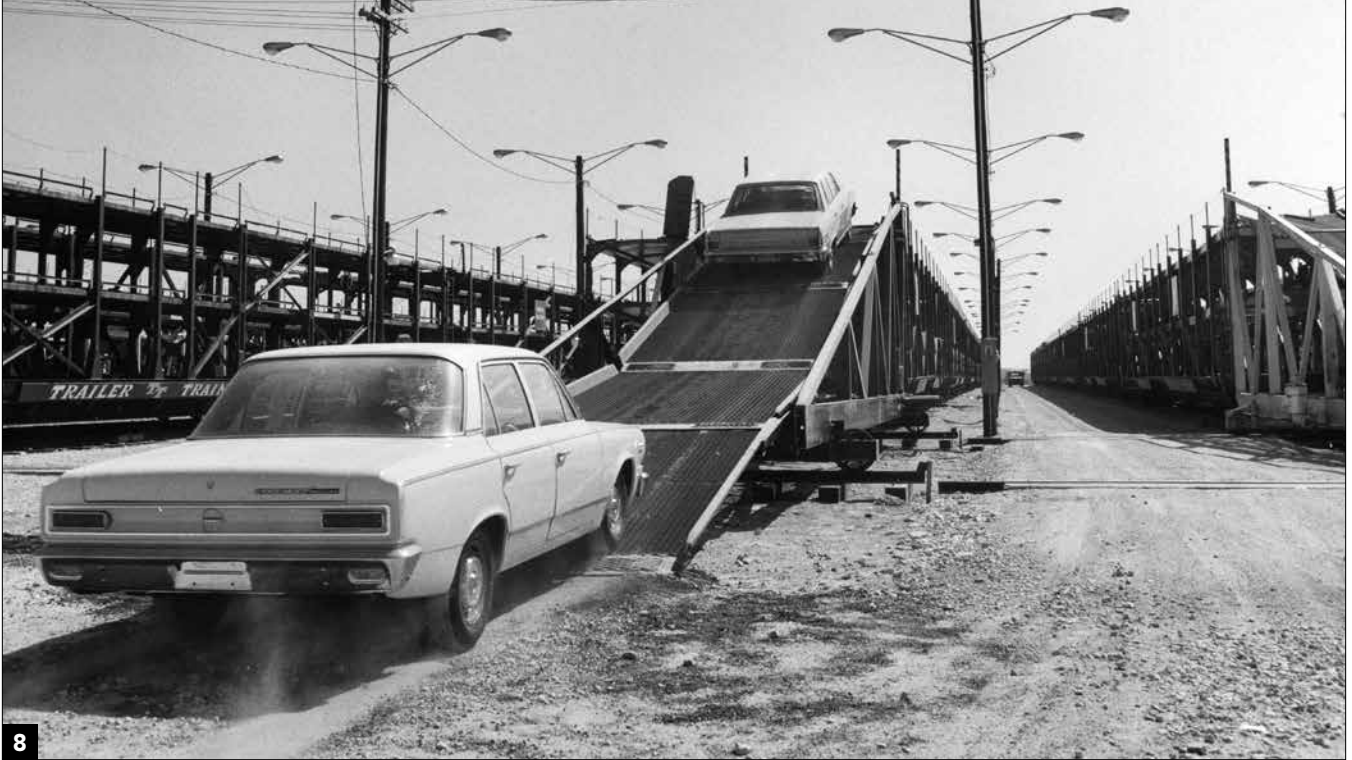
Auto-rack cars allowed easy loading and unloading of multiple cars with end ramps. Here AMC cars are being loaded near Kenosha, Wis., on the Chicago & North Western in 1966. Chicago & North Western, Keith Kohlmann collection
