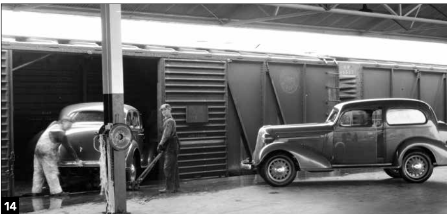
14 Wheeled jacks ("skates") were sometimes used to swing the back end of an auto into position for loading. These are Chevrolets in the late 1930s. Jeff Wilson collection
