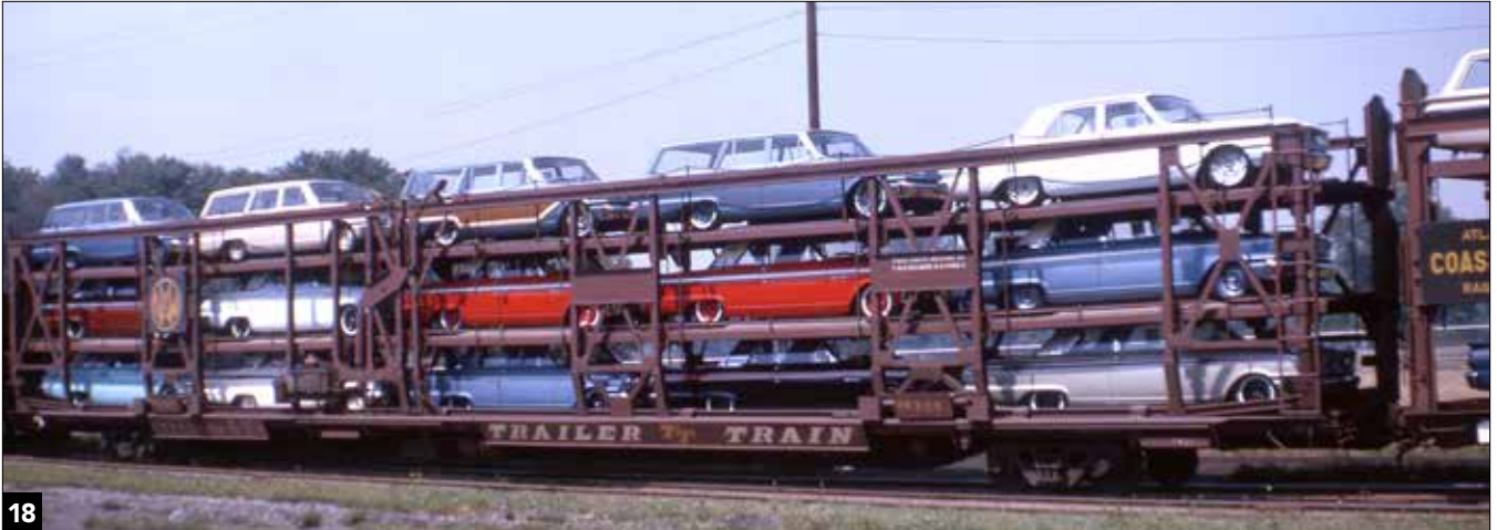
This Whitehead & Kales elevating rack has a different style and pattern of posts and cross bracing compared to the Paragon design. The decks on this Norfolk & Western ETTX car are in the low position. J. David Ingles collection
