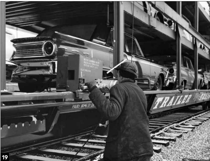
A worker with a power wrench positions the deck of a Pennsylvania Railroad LoHiTri rack. Pennsylvania RR
