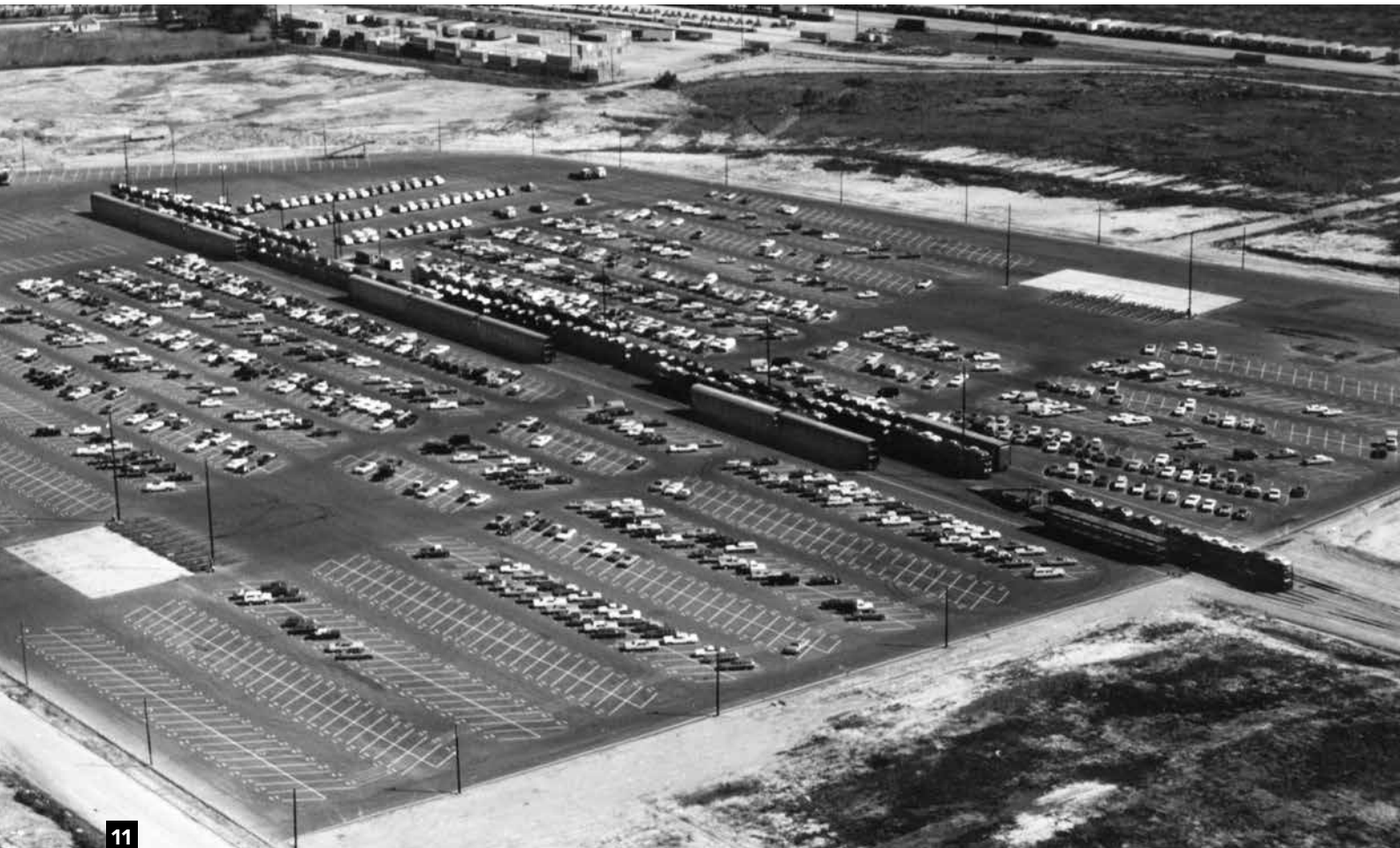
The Santa Fe opened this automobile transload center near Houston in 1976. It has parking for 2,800 vehicles and 36 railcars. Vehicles arriving by rail are reloaded to tractor-trailers for final delivery to dealers in the region. Jeff Wilson collection
