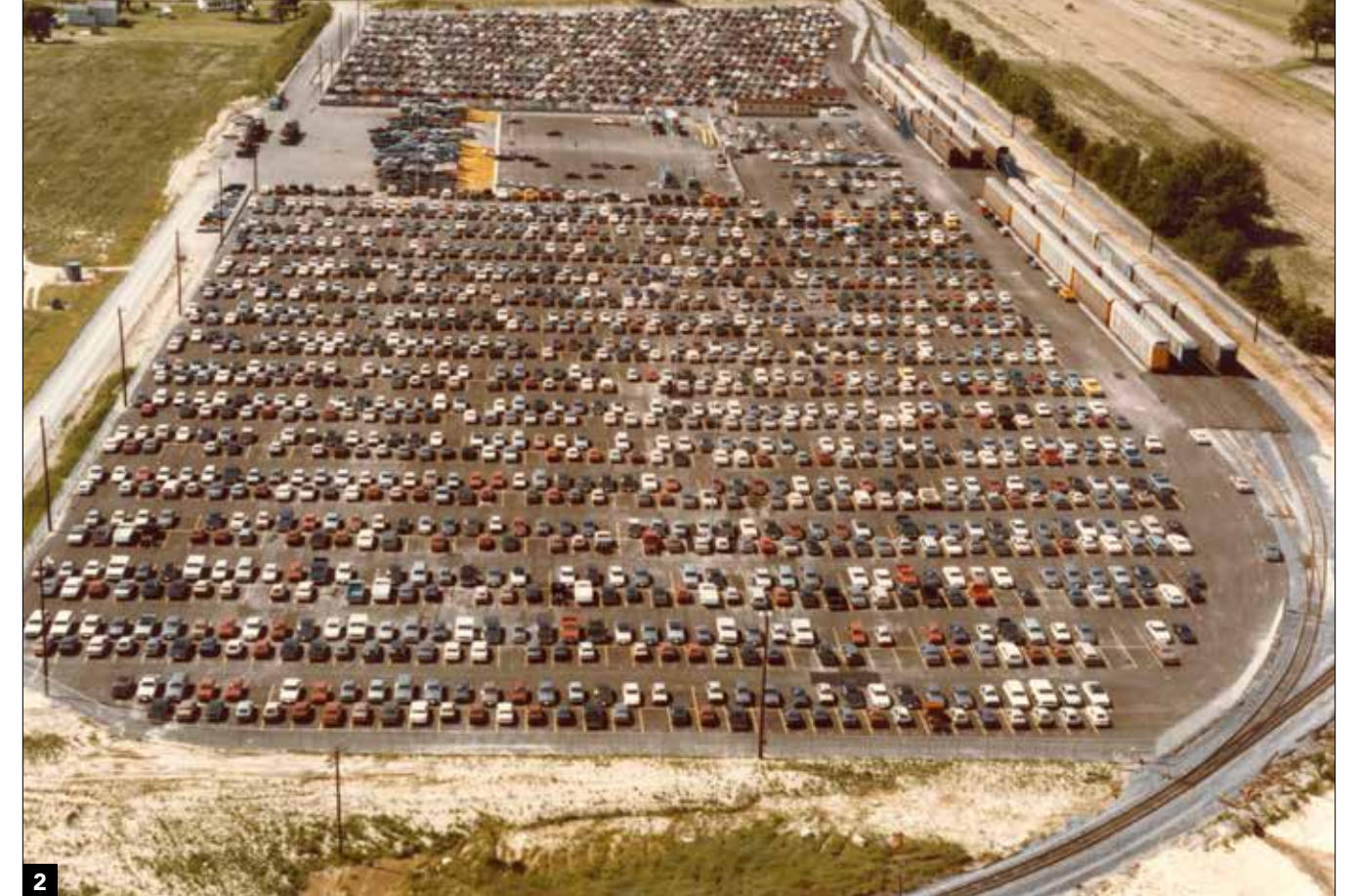
Chessie System's Lordstown, Ohio, transload center represents a typical facility in the 1980s. Three through tracks at right held rack cars, with a large paved, fenced-in parking area and spots for multiple haulaway trailers (yellow ramps toward top left). Chessie System
