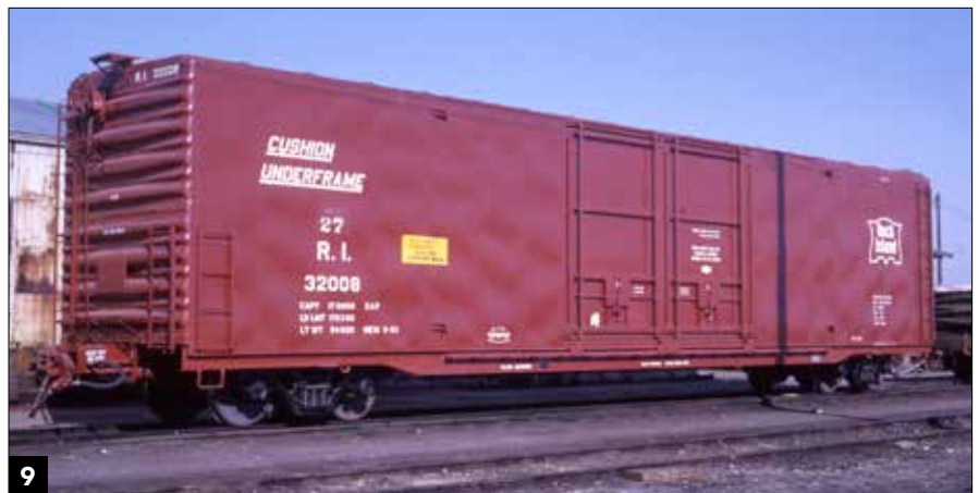
Newly designed 60-foot parts boxcars, like this one from Thrall, began arriving in 1963. Operated in pool service, the "27" above the reporting marks shows the plant assignment of this Rock Island car. J. David Ingles collection
