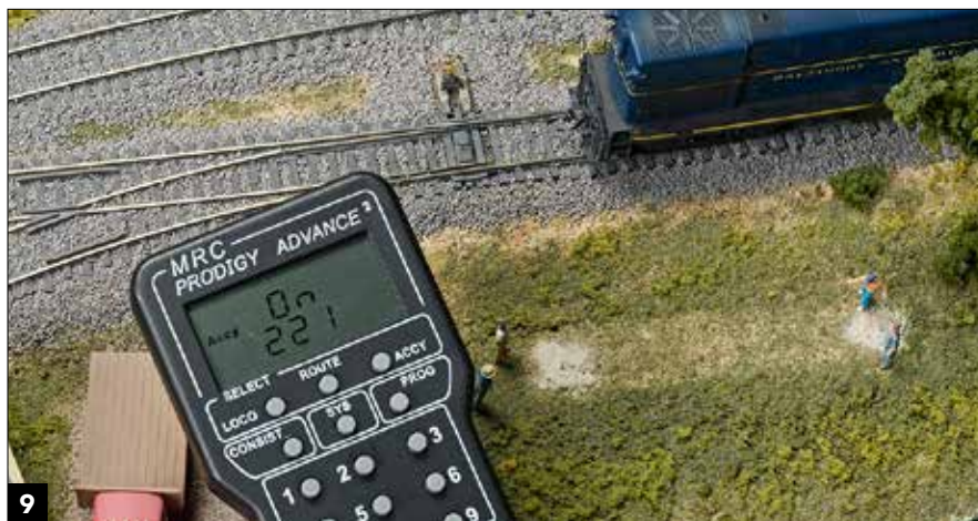
Accessory decoders can control switch machines, as shown above, or many other accessories on a layout.
