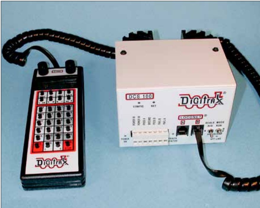
This is the Digitrax DC100 set, with a combined command station and booster (right). The UT400 cab (left) is Digitrax's top-of-the-line unit, and is also available in a wireless (radio) version.
