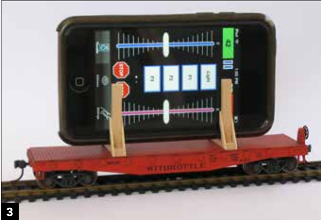
3 WiThrottle can be used to run a layout. The dual throttle app is shown. B. Hoffman
