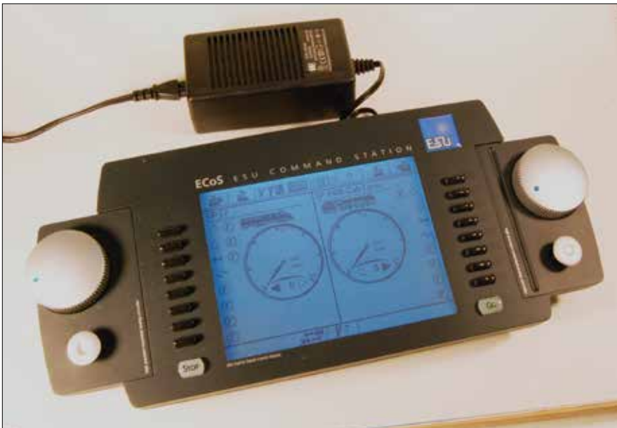
The ECoS system by ESU has several unique features, including a 7" touch screen and the ability to function as a bridge between the rails and another DCC system.
