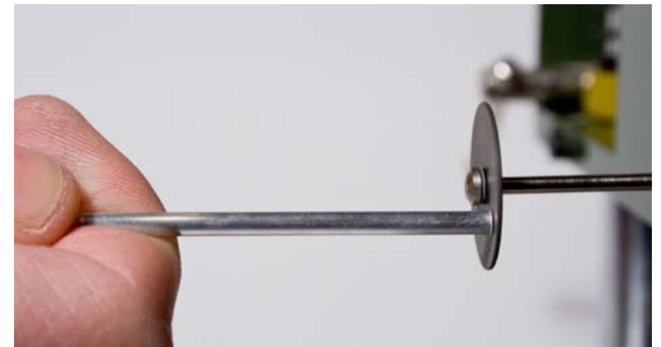
The ends of the pipes are sanded smooth by holding them lightly against a rotating disk cutter.
