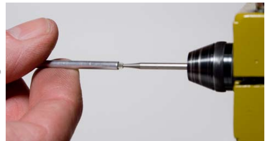
Widening the pipe openings with a high-speed cutter thins the material and gives the pipes a more realistic appearance.
