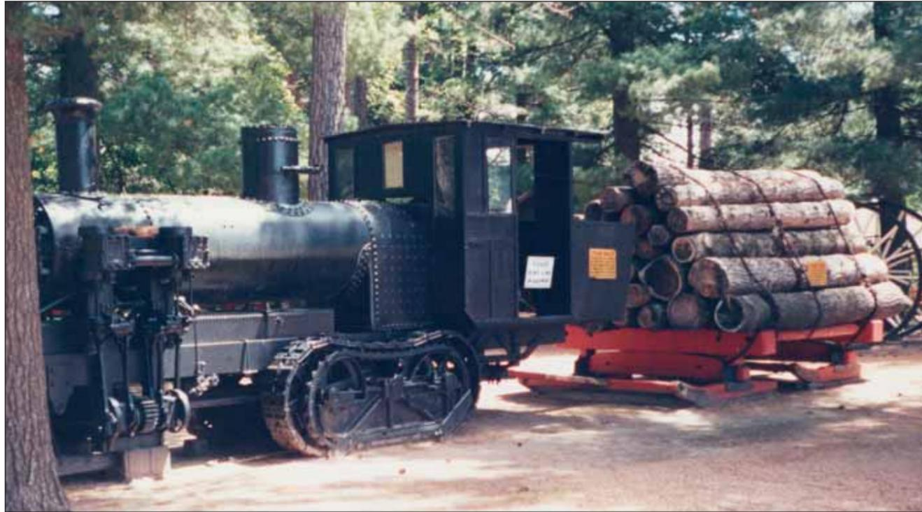
The Lombard Log Loader was a tracked vehicle for hauling logs and sleds on snow. It was steam powered and used a Shay engine.
