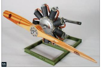
The small, compact engine was dwarfed by the propeller. The 110-horsepower Oberürsel UR.II engine weighed only 330 pounds wet and was 37.7 inches in diameter, the Axial propeller was 8-feet, 7.15-inches in diameter.
