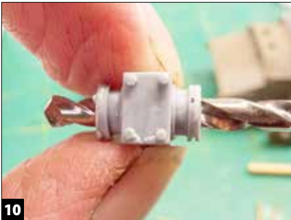
10 In my case some cross drilling was required to allow the brass pins to pass through pivot points.
