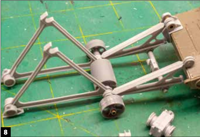
8 Before completing the hull details, I prepared and test-fitted the front arms of the bridge deployment mechanism to ensure everything will line up with the hull-top gearbox and deployment shaft.
