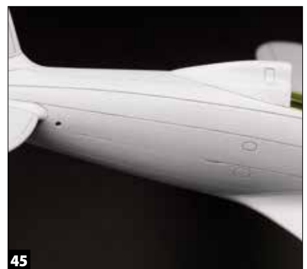
45 Some of the filler along the panel lines, super glue, in this case, chipped. The initial coat of primer revealed it. It wasn't hard to fix, but it was annoying.
