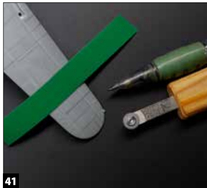
41 Photos show the Saetta's rivets to be visible, even under camouflage, and most of them are double lines. As a compromise for scale, I added single lines and only some of them. I have trouble keeping lines of rivets straight, so I drew guides with a drafting pencil and Dymo tape as a straightedge.
