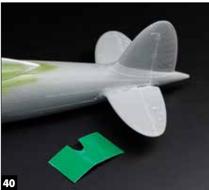
40 I scribed missing panel lines on the rear fuselage. To outline the curved fairings around the stabilizers, I used a template cut from Dymo labeling tape.
