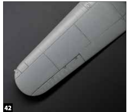
42 After all of the rivets were done and the panel lines were re-scribed, I sanded the airframe and applied a dark wash to check for irregularities. The aileron hinge covers were lost to sanding so I re-scribed them also.
