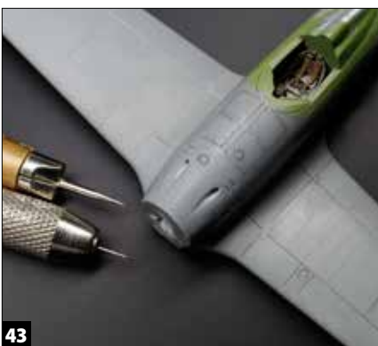
43 I drilled out the gun channels and re-scribed the outlines. I also added various screws using either an Olfa needle (top) or a sewing needle mounted in a pin vise.
