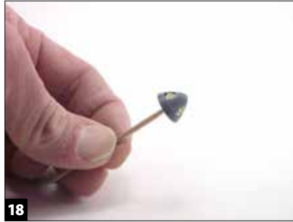
18 A toothpick pushed into the prop shaft hole of this Messerschmitt spinner allows you to easily turn the part for all-around painting.
