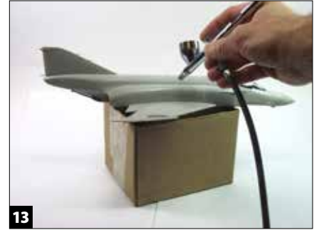
13 Small cardboard boxes can be modified to fit particular models, and they are easy to replace after you cover them with paint.
