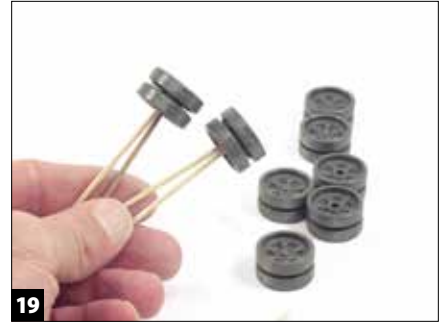
19 If the holes are too big for a single toothpick, as on these T-90 road wheels, try squeezing two toothpicks in; the wood provides enough give to allow a snug fit.
