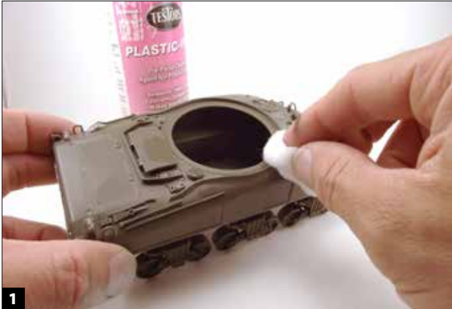
1 Planning to use Tamiya acrylics, I first cleaned the surface using Testors Plastic Prep on a cotton pad to remove any skin oil left on the model during its construction.
