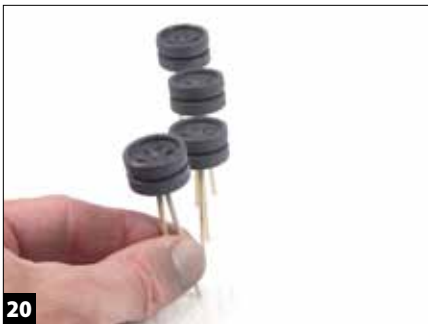
20 Save some foam packaging material to use as drying racks. Foam from around electronics components works well.
