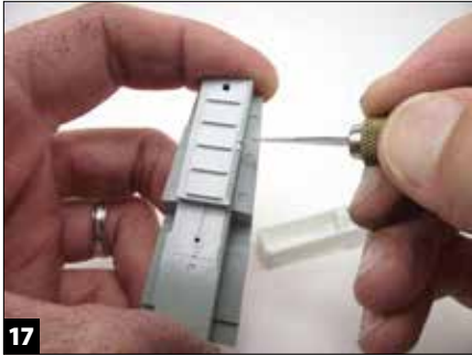
17 Glue and paint don't mix. A No. 11 blade is the perfect tool for scraping paint from the joining surfaces on an area of a wheel well from an F-4 Phantom.
