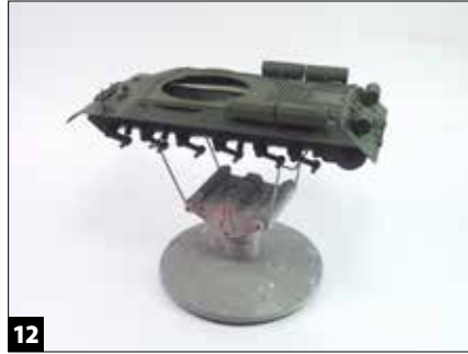
12 Paint stands hold a model steady and allow you to turn it for access and ease of painting.
