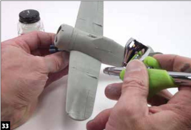
Work slowly and build up the Testors Glosscote in multiple layers to produce a glass-smooth surface.
