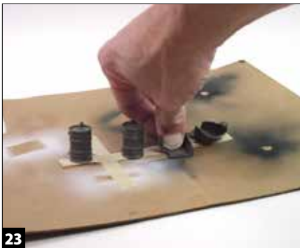
23 Double-tape pieces, such as this collection of T-90 details, to cardboard for painting. I keep a supply of scrap cardboard at my workbench.
