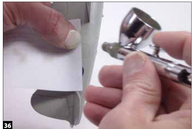
Holding a piece of paper over the decal, I touched up the spot with light gull gray sprayed at 15 psi.
