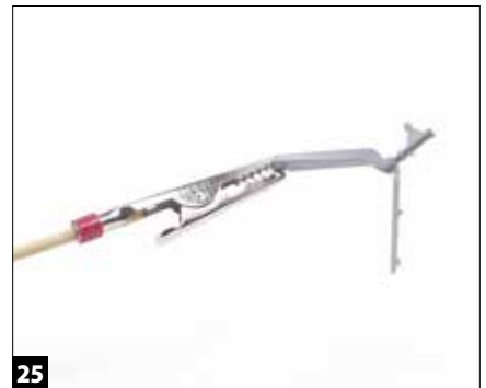
25 You can find alligator clips with other electrical supplies. The round wire holder is about the perfect size to hold a wooden skewer.
