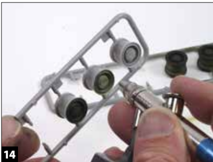
14 A convenient option, sprue makes a terrific handle for airbrushing parts. It's almost like they planned it that way.
