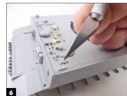
6 I used the tip of a new No. 11 blade to maneuver small parts such as headlight bases into position. You don't have to press hard, just enough to pick up the piece.
