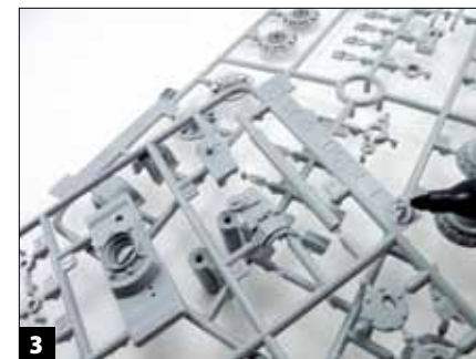
3 I highlighted the sprue designations with a marker to make finding parts easier.
