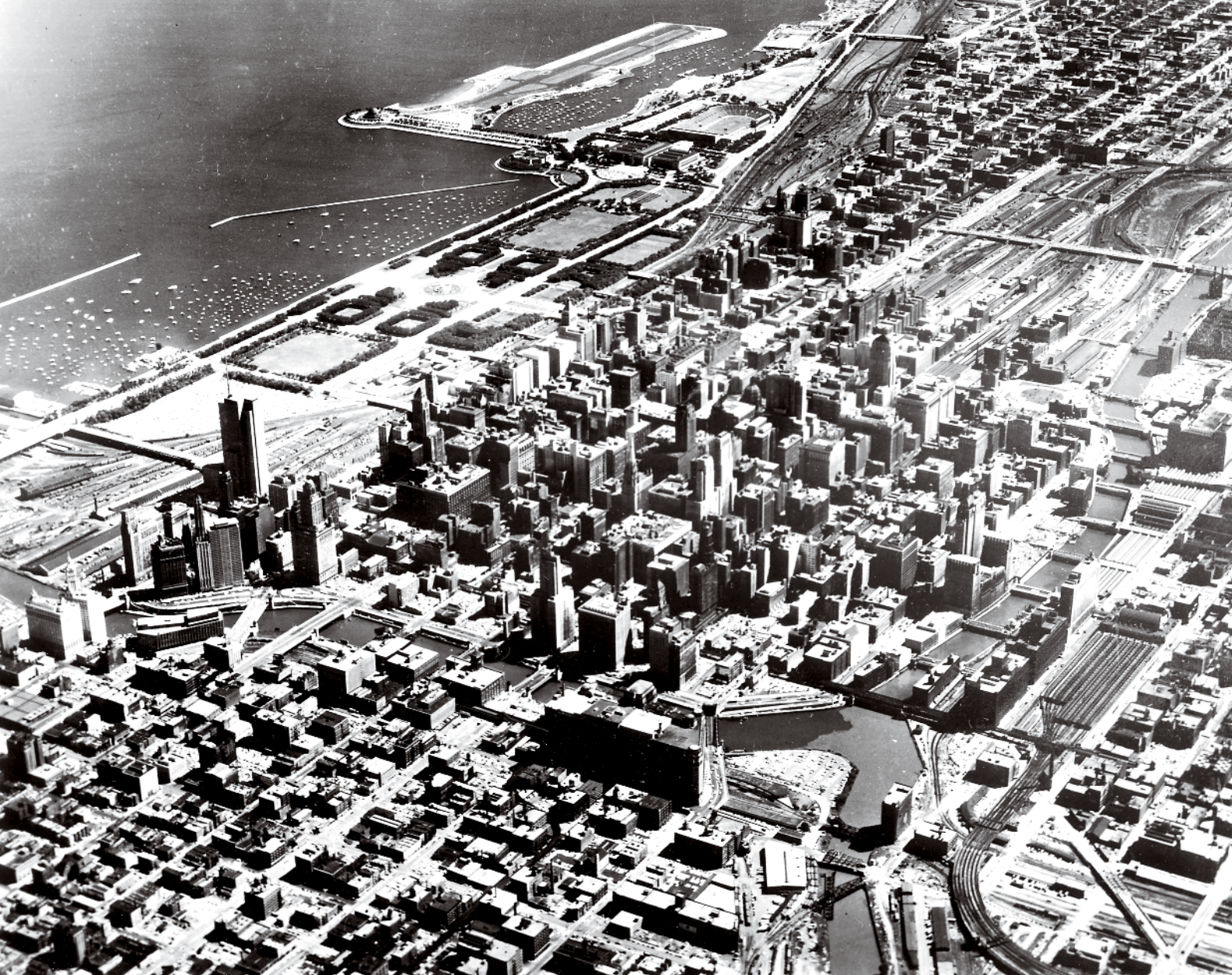
Chicago's central business district in 1962 shows passenger stations abutting the core on the south and west, and coach yards and freight houses occupying valuable land. Only six streets skirted or penetrated the tracks to the south. The warehouse-lined north and south branches of the Chicago River meet at lower right.
