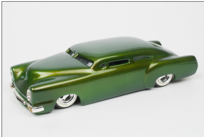
Ken Brickell's 1951 Chevrolet Custom is low and smooth, with a chopped and sectioned body, and he also added quad headlights. The paint is a clever Flip Flop green enamel.
