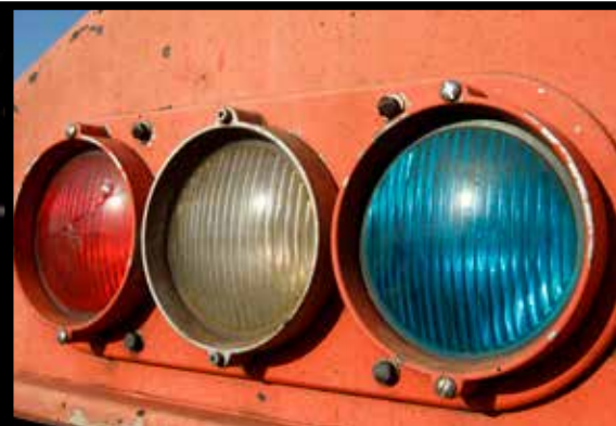
Custom CN features on the first order included nose-mounted class and marker lights as on No. 2413.
