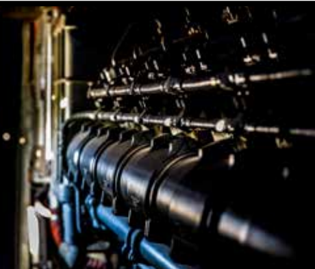
Heart of the matter: 7FDL-16 prime mover nestled in the full-width cowl carbody of CN 2401.
