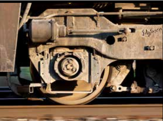
All 84 Dash 8-40CMs built rode on MLW-Dofasco designed ZWT-3 high-adhesion trucks.
