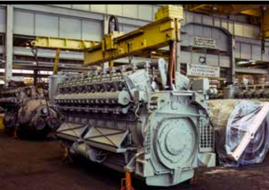
7FDL-16 prime mover and CMG 194 main alternator destined for Dash 8 installation, Building 10, Erie, Pa.
