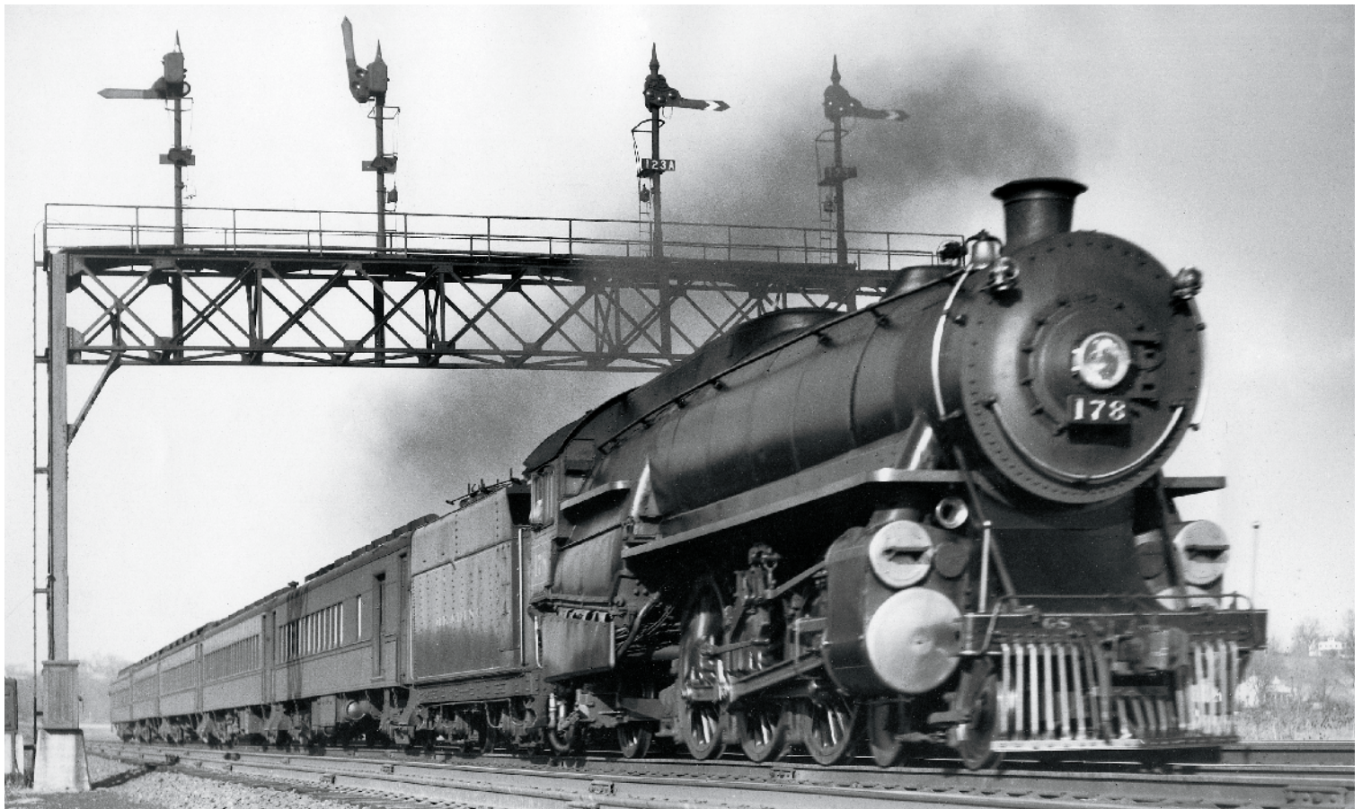
The semaphore blade has already begun to fall as Reading G-2sa Pacific 178 sweeps under the signal bridge near Glen Moore with a New York-Philadelphia express. In common with Delaware & Hudson, Reading became interested in clean-lined English engines and, as a result, semi-streamlined two Pacifics. Say, is that a horn tucked under the running board?
