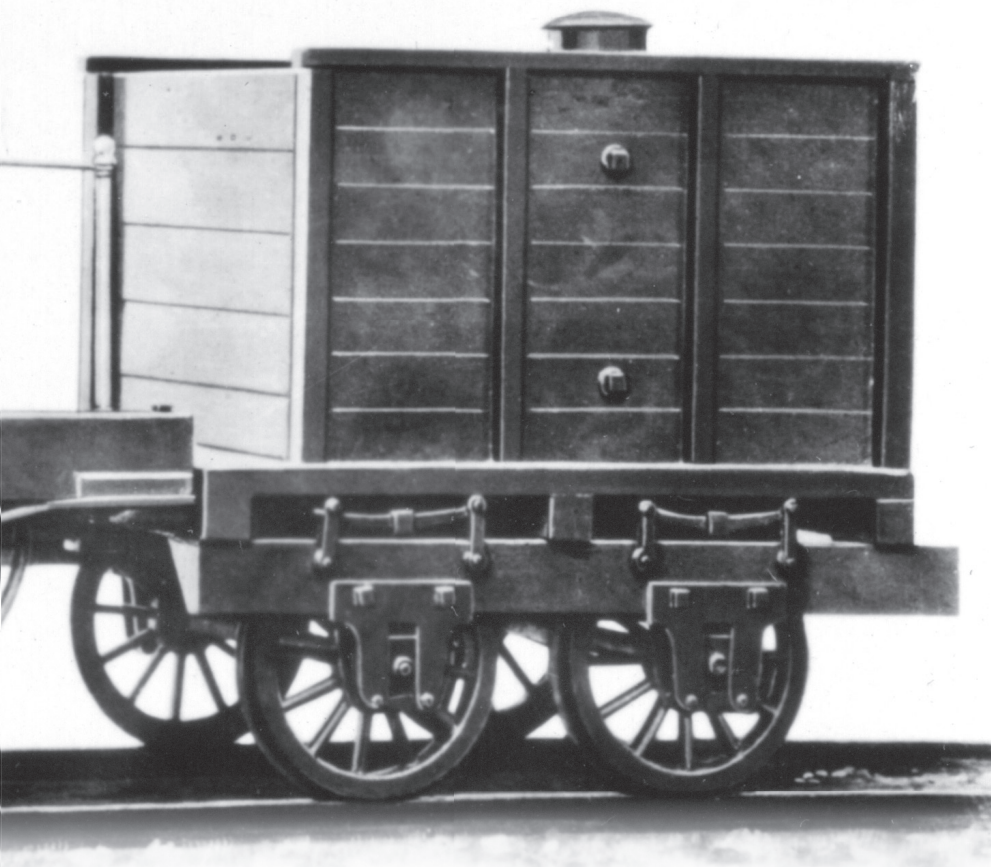
Old Ironsides , designed and built by Matthias Baldwin, made its first run in 1832 on the Philadelphia, Germantown & Norristown Railroad. The 5-ton locomotive was among the first steam locomotives built in the United States, and the first built by Baldwin. The rear (54" diameter) driving wheels powered the engine, which was technically a 2-2-0 under the Whyte system. Trains magazine collection
