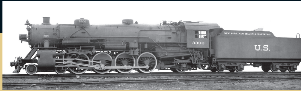
The USRA in 1919 assigned 10 light 4-8-2s to New Haven. The railroad liked them enough to order 39 additional copies during the 1920s. Alco
