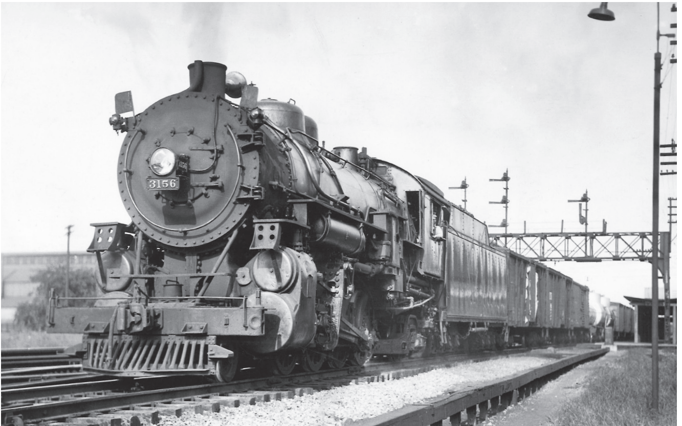
An Erie 2-8-2 leads Extra No. 3156 West out of Marion, Ohio. No. 3156 is one of 40 Class N-3 Mikes (Nos. 3155-3194) built by Baldwin for the Erie in 1923. They were retired around 1950. H. W. Pontin photo
