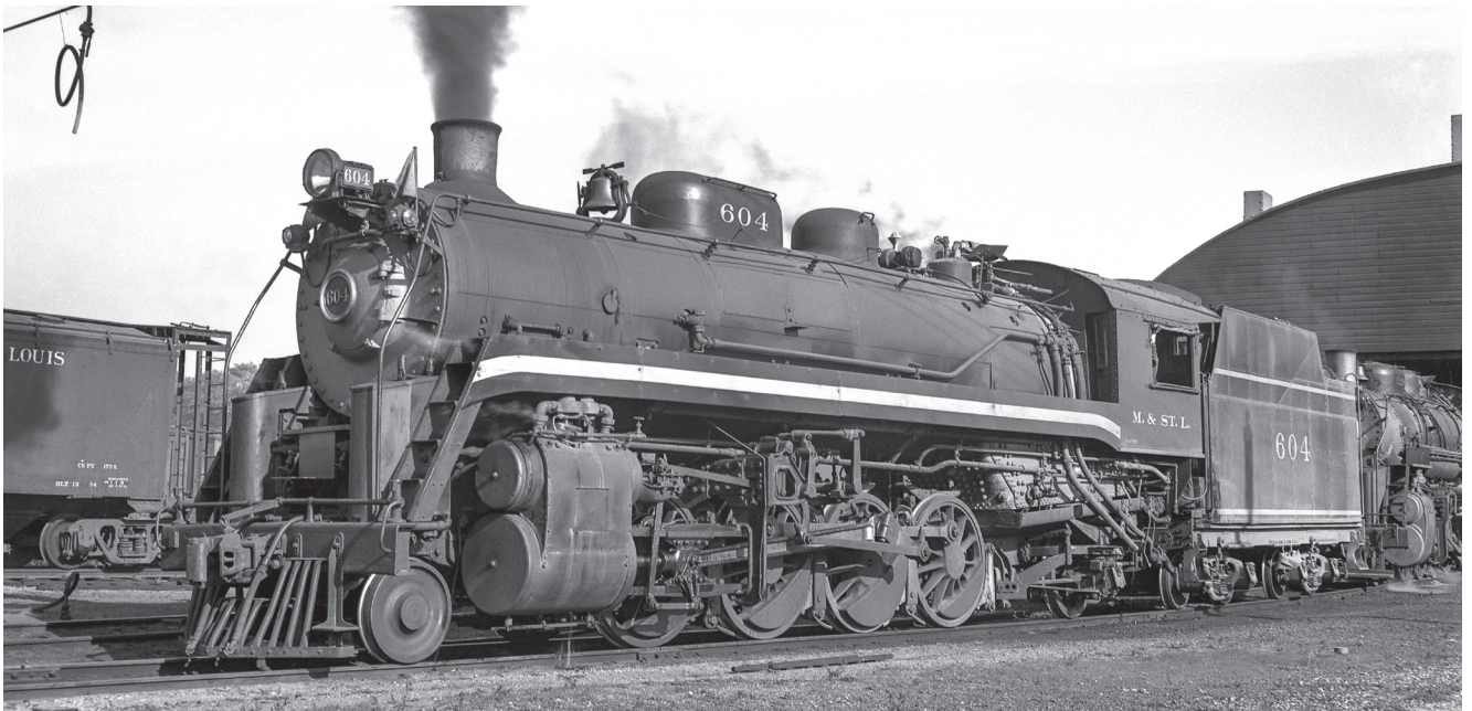
Minneapolis & St. Louis 2-8-2 No. 604 rests at Peoria, Ill., on Oct. 12, 1947. Between 1915 and 1921, M&StL bought 35 unusually light Mikados from Alco. They weighed between 252,500 and 259,000 pounds with 20x30-inch cylinders and 59" drivers. John E. Pickett collection
