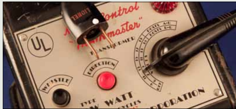
By painting a small white dot next to the left blade of a plug, you'll know how to insert it correctly into the wall socket.
