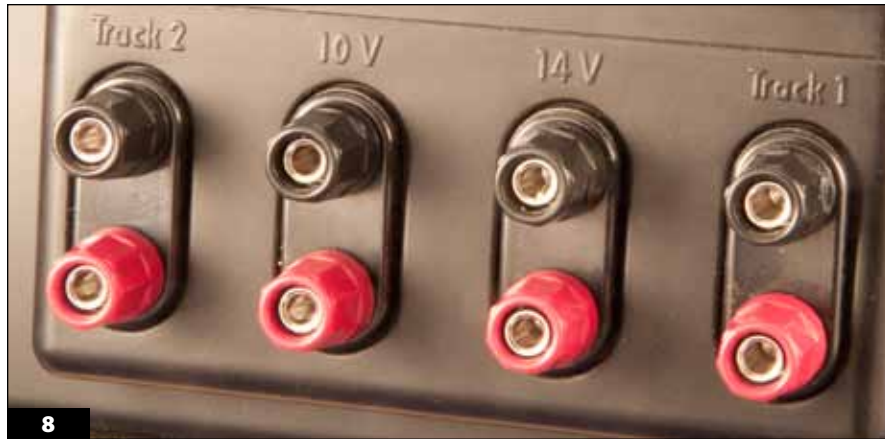
8 The power posts on this modern transformer are clearly identifiable by their red color.
