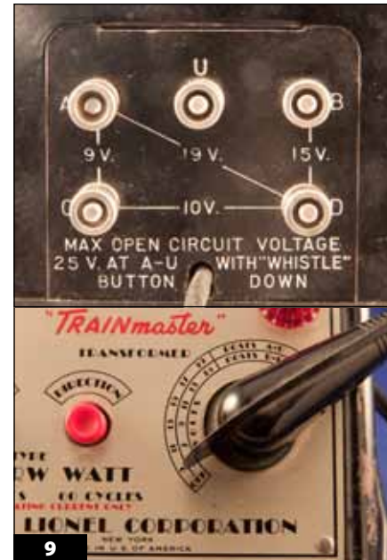
9 On the back of this Lionel RW Transformer (top), the letter U designates the throttle. On the top of the transformer, the label on the throttle dial shows the voltage available with posts AU and BU.
