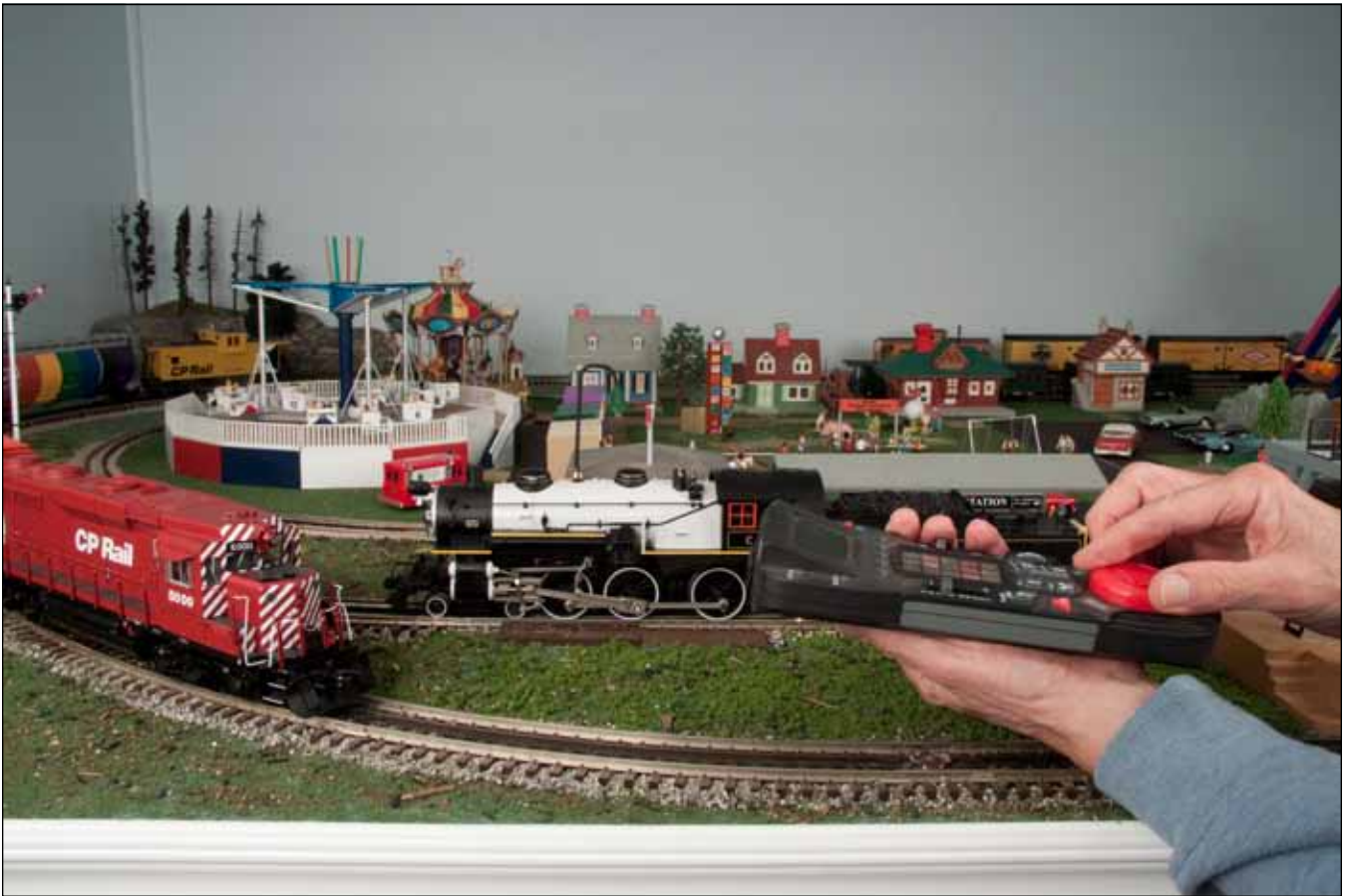
Two or more trains will operate independently on the same track with a command control system, as shown by these trains in Lionel's Legacy line.
