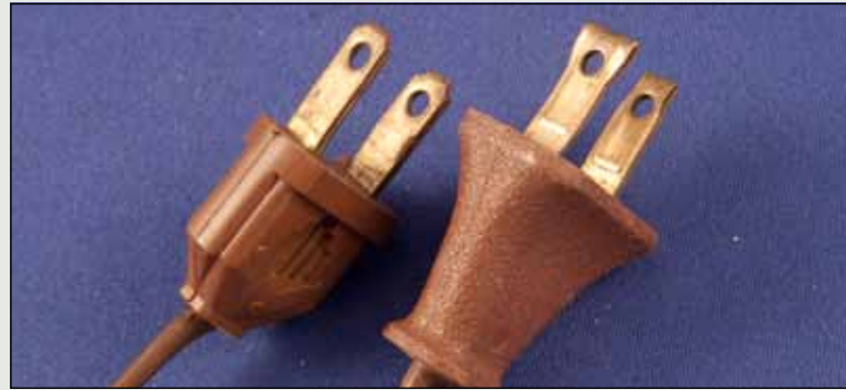
Modern transformers have polarized wall plugs (right) with one blade wider than the other. They can only be plugged into a wall socket one way. Vintage transformers do not have polarized plugs (left) and can be inserted into a wall socket with either blade in either slot.
