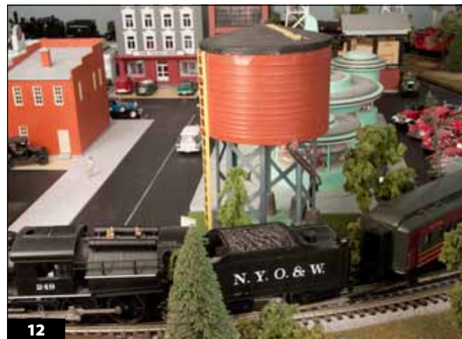
12 Filling the tender with water, pre- and postwar American Flyer style, takes place as a solenoid lowers the spout with the push of a button.
