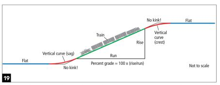
An article by Van S. Fehr, "Understanding vertical curves," appeared in *Model Railroad Planning 2016*. The article describes procedures for calculating and constructing vertical grades. For good appearance, use vertical curves no shorter than the coupler-to-coupler length of the longest equipment and twice as long if possible.
