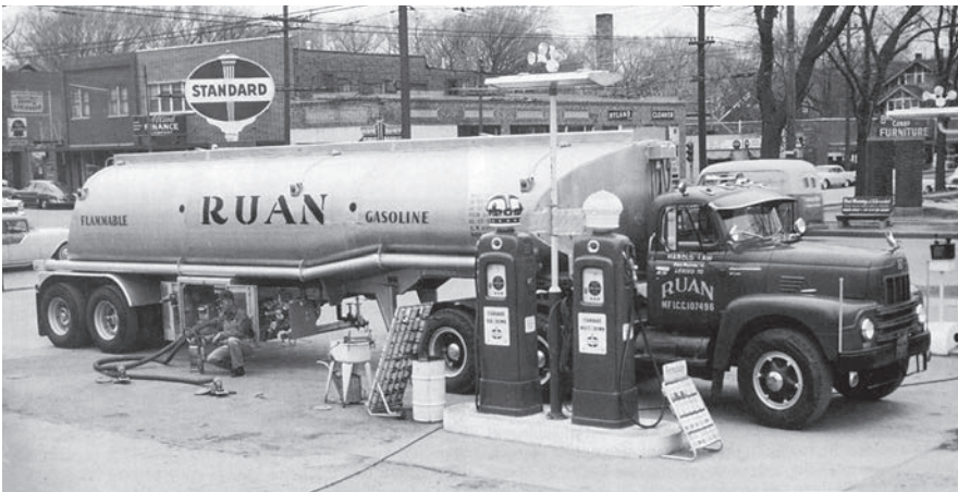
This Ruan trailer typifies large delivery trailers from the late 1950s through the 1960s, with broad, rounded nose (to allow clearance to a close-coupled cab), side-mounted hose and control connections, and simple, curved mud guard over the wheels. This truck is making a delivery to a Standard station in Iowa in 1957. Ken Scarpino; Mont Switzer collection
