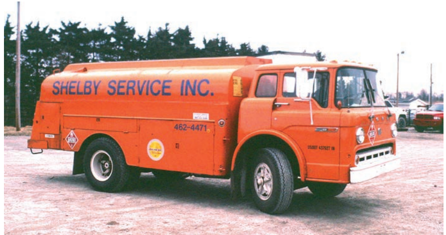
Shelby Petroleum in Greenfield, Ind., operated this delivery truck with a Ford C cabover chassis in the 1980s. The modern-style tank lacks the side platforms of earlier tanks, since modern loading racks allow direct roof access.
