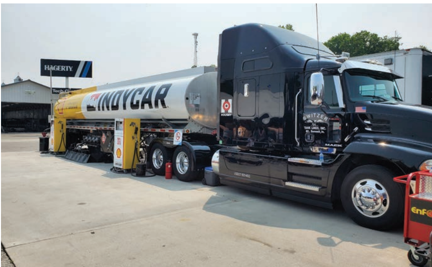
This modern Switzer Tank Lines semi is set up as a portable station to provide fuel for races. It's at Elkhart Lake, Wis., in 2023. Note the side reflective striping, side-mounted delivery connections, top rub rails, and flatter nose compared to earlier trailers. Mont Switzer collection
