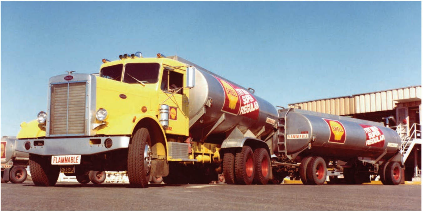
To maximize payload while complying with length/weight restrictions, a common setup for transport trucks in California was a large tandem-axle straight truck pulling a trailer. This Shell tank rides on a Peterbilt chassis in the 1970s. Jeff Wilson collection
