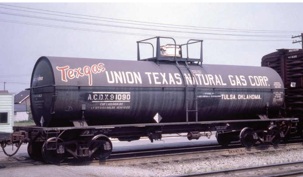
General American built this 11,000-gallon pressure car in 1955. The ICC 105A 300W car is carrying LPG for Union Texas Natural Gas Corp., a division of Allied Chemical. J. David Ingles
