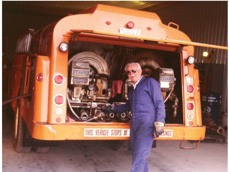
The back compartment houses meters, pumps, and control equipment. The flip-up rear door provides protection to the equipment and operator in bad weather. Mont Switzer collection
