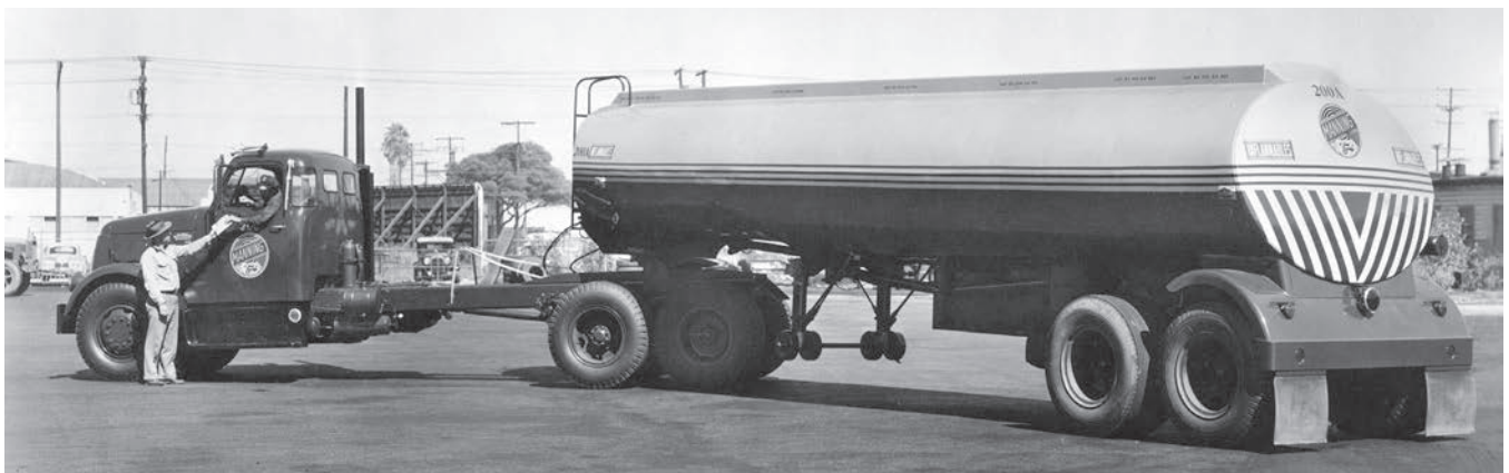
Weight regulations regarding length in some states resulted in semi tractors with extended frames, such as this 1950s-era truck. Modeling features like this can greatly increase realism by matching prototype practice in specific states, regions, and eras. Jeff Wilson collection
