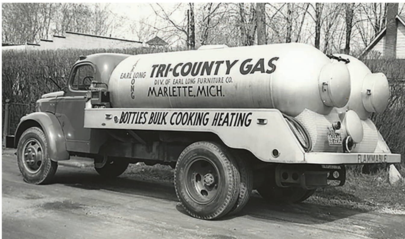
Early LPG trucks often had pairs of tanks side-by-side on the truck chassis. Dealers often sold and serviced appliances and furnaces, as well. Mont Switzer collection
