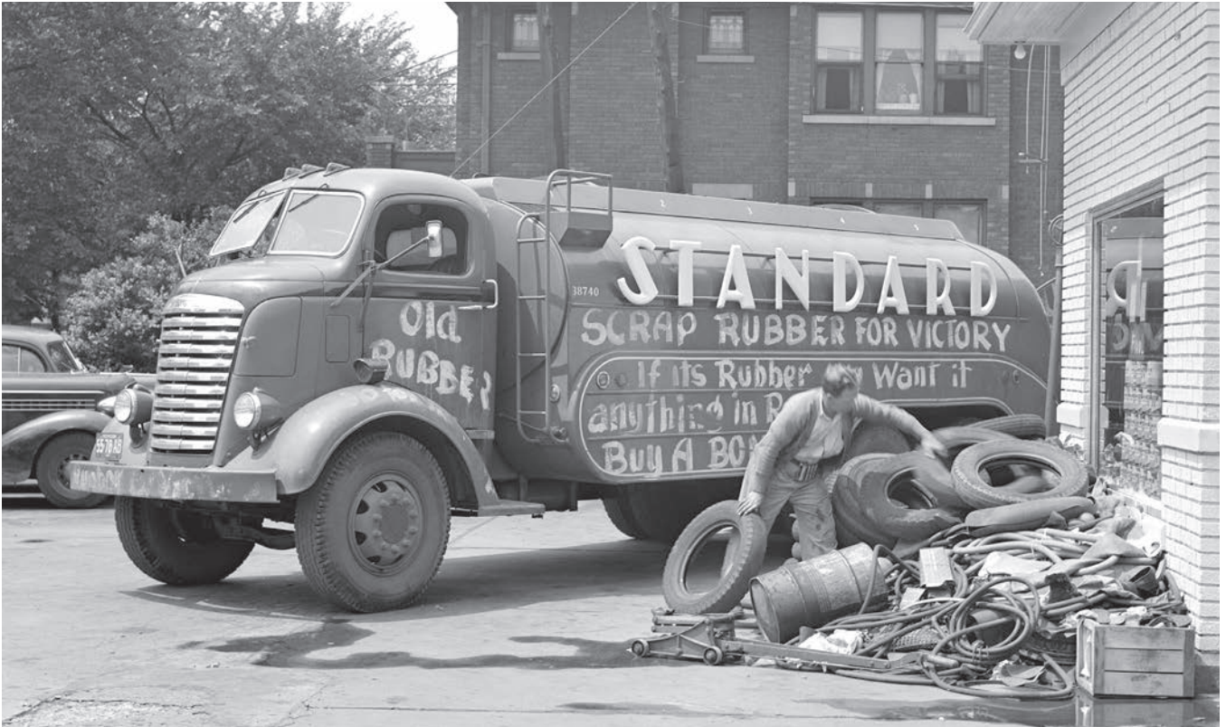
Streamlining was coming to fuel truck bodies by the late 1930s. This Standard tank, on a tandem-axle GMC chassis, has side sheathing and distinctive stand-alone side lettering. The dealer is leading a scrap rubber drive near Detroit in 1942, with temporary lettering on the cab and tank sides. Arthur S. Siegel, Library of Congress
