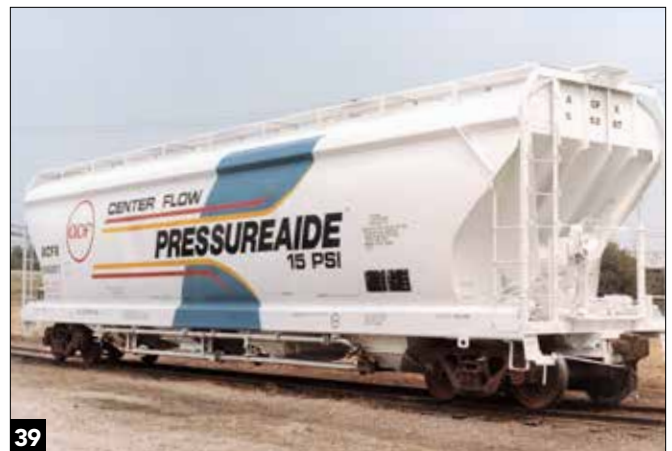
Pressureaide cars look like standard Center Flows, but with two sets of piping along the sides of the outlet bays. ACF Industries
