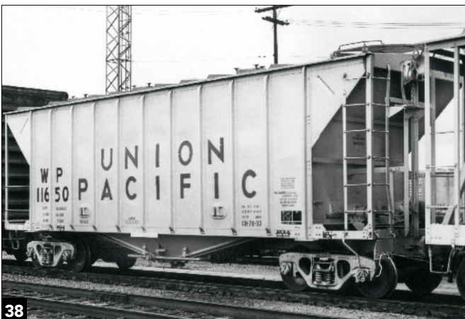
Single-bay Airslides had open end platforms. Post-1965 cars like this 1966-built Union Pacific car had triangular end fillets, even though there was no slope sheet behind them. Jim Hediger
