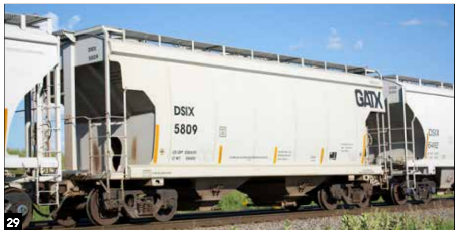
29 This NSC 3220 has squared-off notches for ladder mounting at each end. The sill continues straight at the end platforms. The car was built in 2006. Cody Grivno
