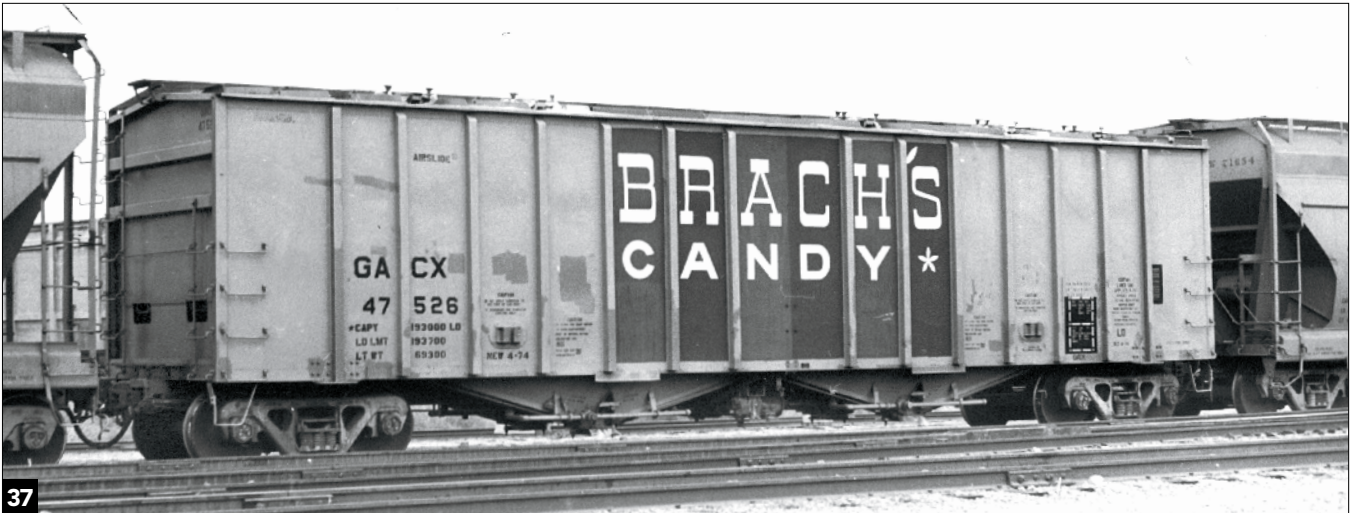
This 4,180-cf, two-bay Airslide was built in 1974. The box-like cars have longitudinal outlet bays. Note the solid ends with horizontal braces and two rectangular lower cutouts. Jeff Wilson collection
