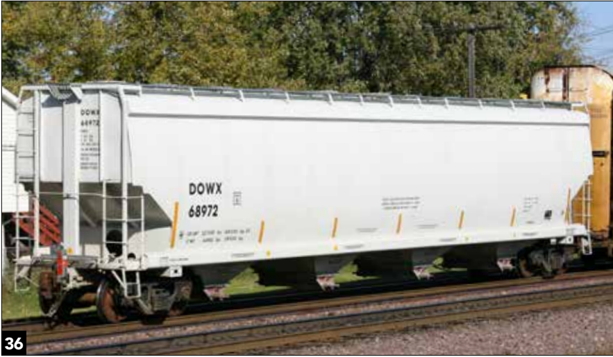
Among National Steel Car's latest offerings is this 6,245-cf plastics car. Note the large vertical brace centered on the end and the small notches at the top ladder rung. Jeff Wilson
