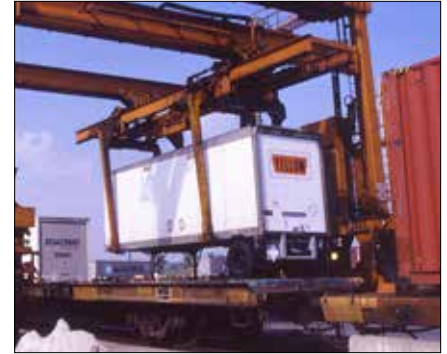
For a trailer lift, the crane operator lowers the arms, adjusts the spread to match the trailer size, and engages the lower clamps on the lower side rails. The trailer is then lifted and placed on the ground and the clamps and arms disengaged.
