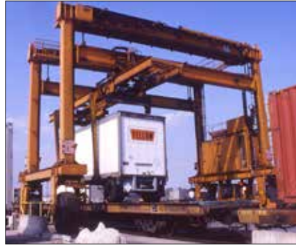
For a trailer lift, the crane operator lowers the arms, adjusts the spread to match the trailer size, and engages the lower clamps on the lower side rails. The trailer is then lifted and placed on the ground and the clamps and arms disengaged.
