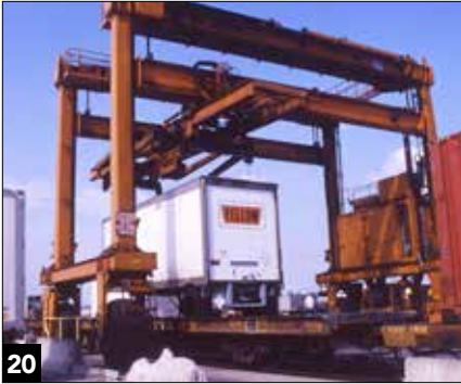
For a trailer lift, the crane operator lowers the arms, adjusts the spread to match the trailer size, and engages the lower clamps on the lower side rails. The trailer is then lifted and placed on the ground and the clamps and arms disengaged.
