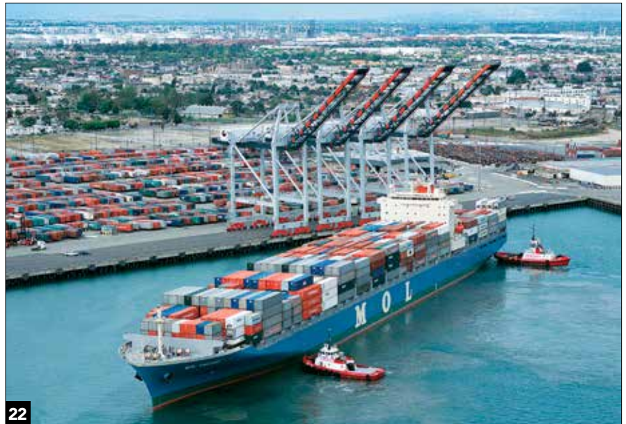
Tugboats guide the 4,500-TEU Mol Encore (built in 2003) to a berth with multiple unloading cranes at the Port of Los Angeles. The port features 270 berths with 91 ship-to-shore container cranes. Port of Los Angeles
