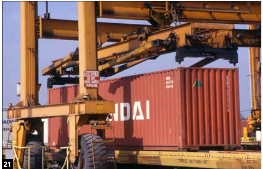
For a container, the operator matches the crane's pins to the corner castings. Doing a pair of end pins first ensures that the other end will match when lowered.
