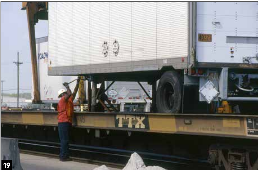
A ground crew member works in tandem with the crane operator. Here, a worker lowers the trailer landing gear and unlocks the hitch to release the kingpin before the crane lifts the trailer.
