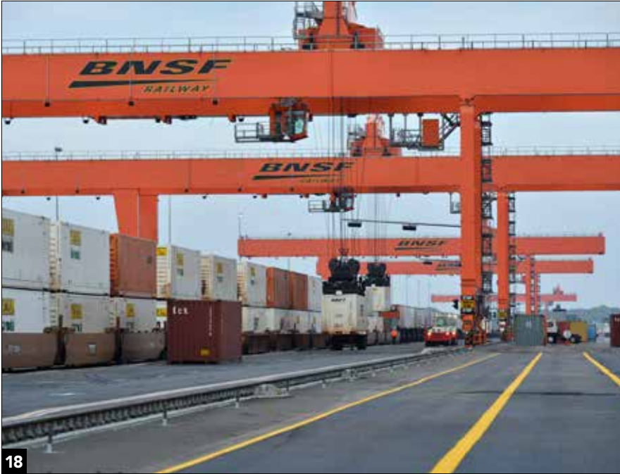
The five cranes at BNSF's Logistics Park Kansas City stand 90 feet tall, ride on rails, and are electrically powered. Each can work multiple tracks, or multiple cranes can work the same train. BNSF
