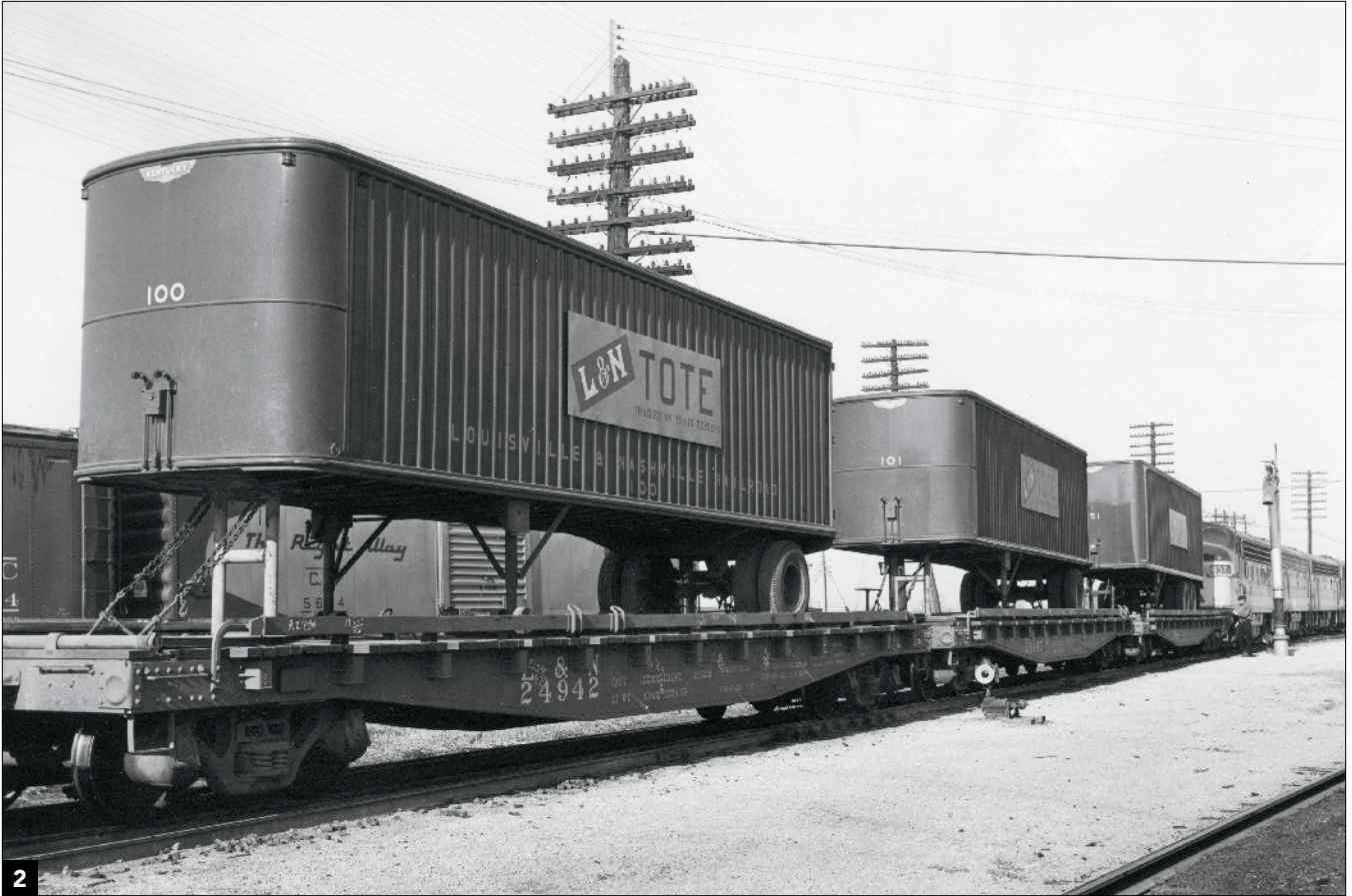
Louisville & Nashville converted these 43-foot flatcars for TOFC service in 1955 by adding rub rails and jack connections. Kentucky built the exterior-post 32-foot trailers. Louisville & Nashville
