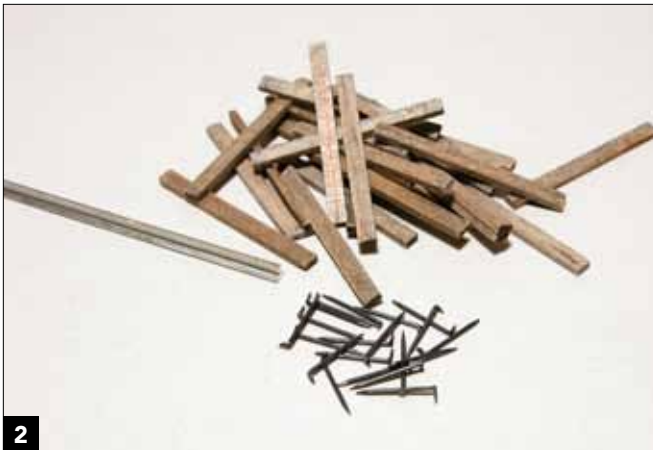
2 The components needed for handlaying track are rail, ties, and spikes.
