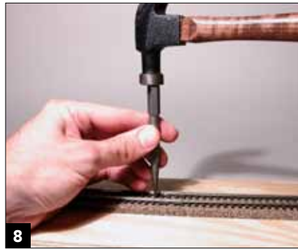
Use a nail set to finish driving the track nail below the railhead level.
