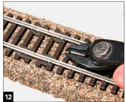
Wire cutters or rail nippers work well for grabbing track nails that need to be removed. Carefully work the jaws under the nail head.
