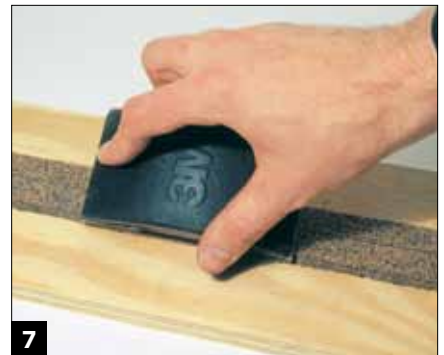
7 Use a sanding block with coarse or medium sandpaper to remove the rough edge.
