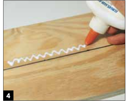
4 Run a bead of white glue along one edge of the centerline and then press the cork into place.
