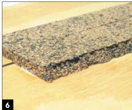
6 One side of the cork usually has a rough burr along the top edge where it was connected to its mating piece.
