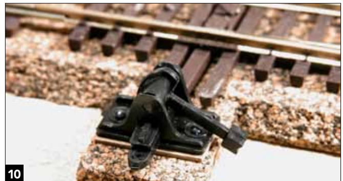
Caboose Industries ground throws work well and are closer to scale than side-mounted controls. This one is mounted on an HO Atlas turnout.
