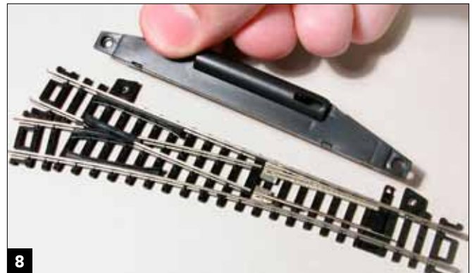
Removing the control on this Atlas N scale code 80 turnout also removes several tie ends.
