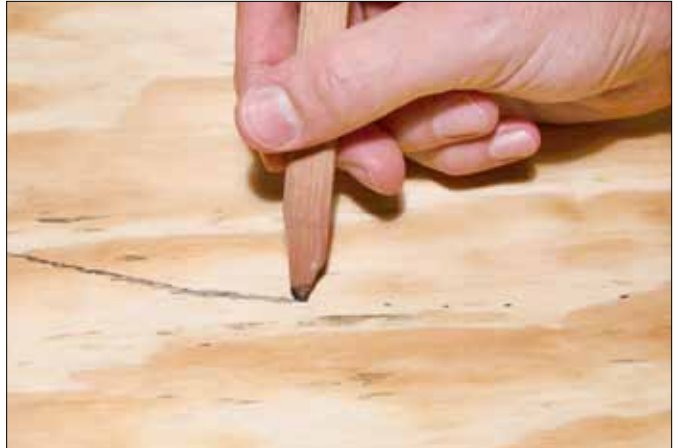
Mark the track center between ties every few inches (left). Then remove the track and connect the dots to mark the centerline.
