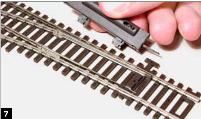
Some manual controls are held by screws, while others, like this Atlas HO code 83 model, snap in place.
