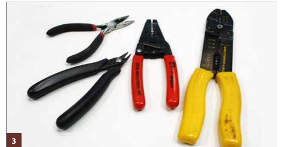
3 Good-quality pliers, wire cutters, and a wire stripper are essential tools for installing wiring.
