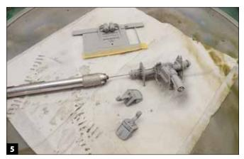
I prepped the individual interior components with Tamiya primer using an airbrush.
