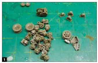
I kicked off by making the wheel assemblies. With 20 units required, each consisting of four parts each, this was a tedious task, but there were no issues here. Just be aware that one wheel on each side fits straight into the hull part and does not need to be assembled as a complete bogie. The drive and idler sprockets were also completed at this stage and put aside for later.
